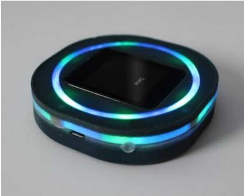
Figure 1.1: Actibles are a smartwatch-based active tangibles platform that incorporates additional sensors to detect stacking and neighboring, as well as LED feedback. The image shows an assembled Actible.
