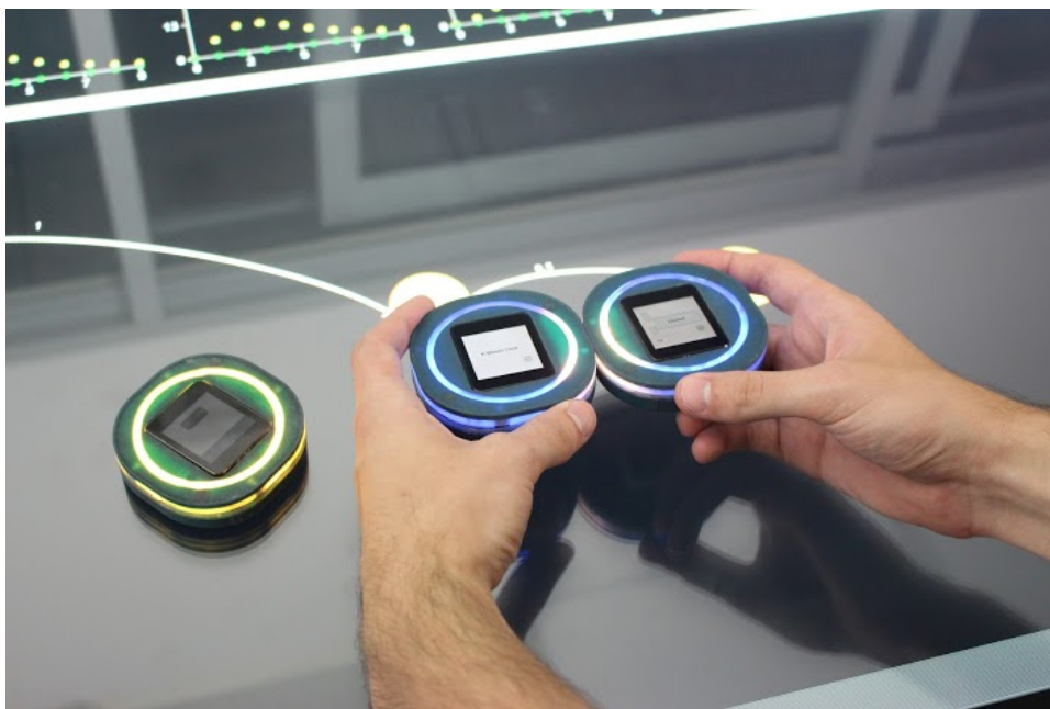
Figure 5.1: The Actibles represent molecules in the Active Pathways system. Off-table neighboring interactions are used to construct reactions between molecules.
