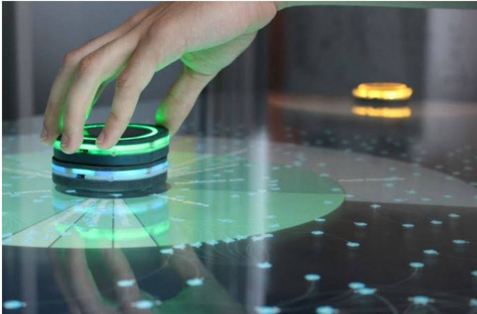
Figure 5.2: Actibles are used to browse gene interaction networks in the Sparse Tangibles system. Stacking one Actible on top of another filters the data associated with the bottom Actible based on the parameters set on the upper Actible.
