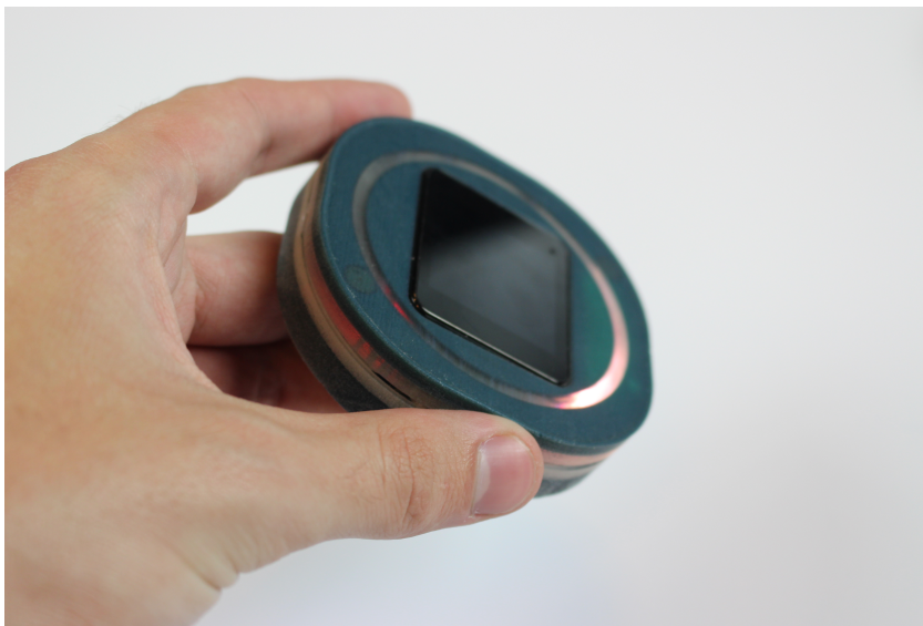
Figure 3.1: The tilt interaction. The tilted edge gives a confirmation flash.
