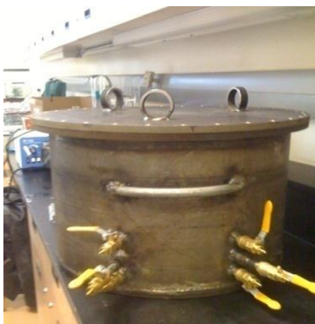
Figure 3. Steel cylinder that houses peristaltic pump. 3 Inlet valves (for spike solutions) are on the right side of the cylinder and 3 outlets to the sampling chamber are on the left side.
