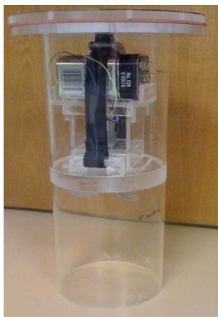
Figure 1. A sampling chamber fully sealed. Top compartment contains 9V battery to power stirrer motor (underneath battery). Bottom compartment is where water samples will be taken.
