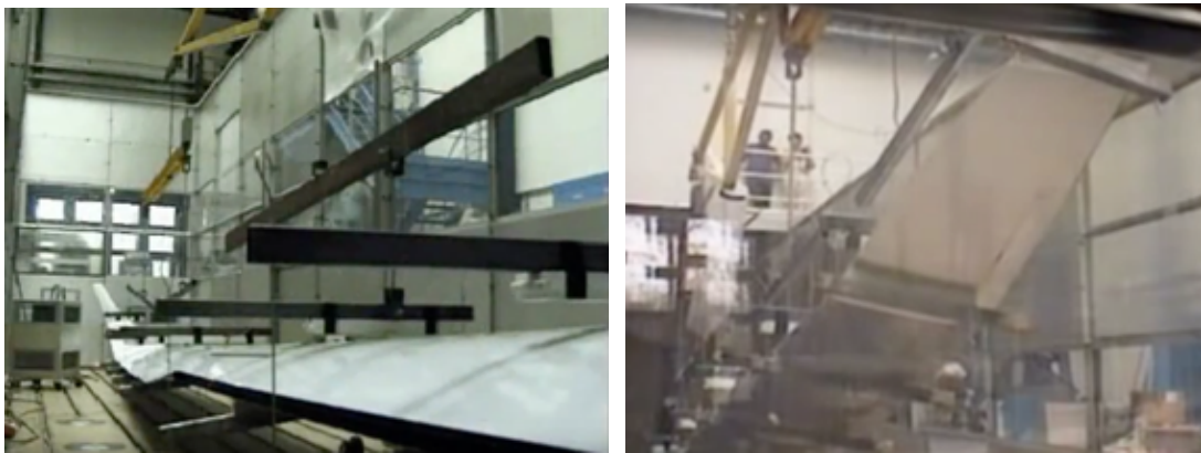
Figure 2-9: DG Flugzeugbau DG-800/1000 wing loading test setup [16]
