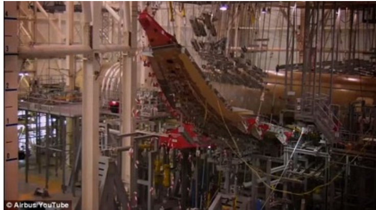
Figure 2-7: Airbus A350 XWB wing loading test setup [16]
