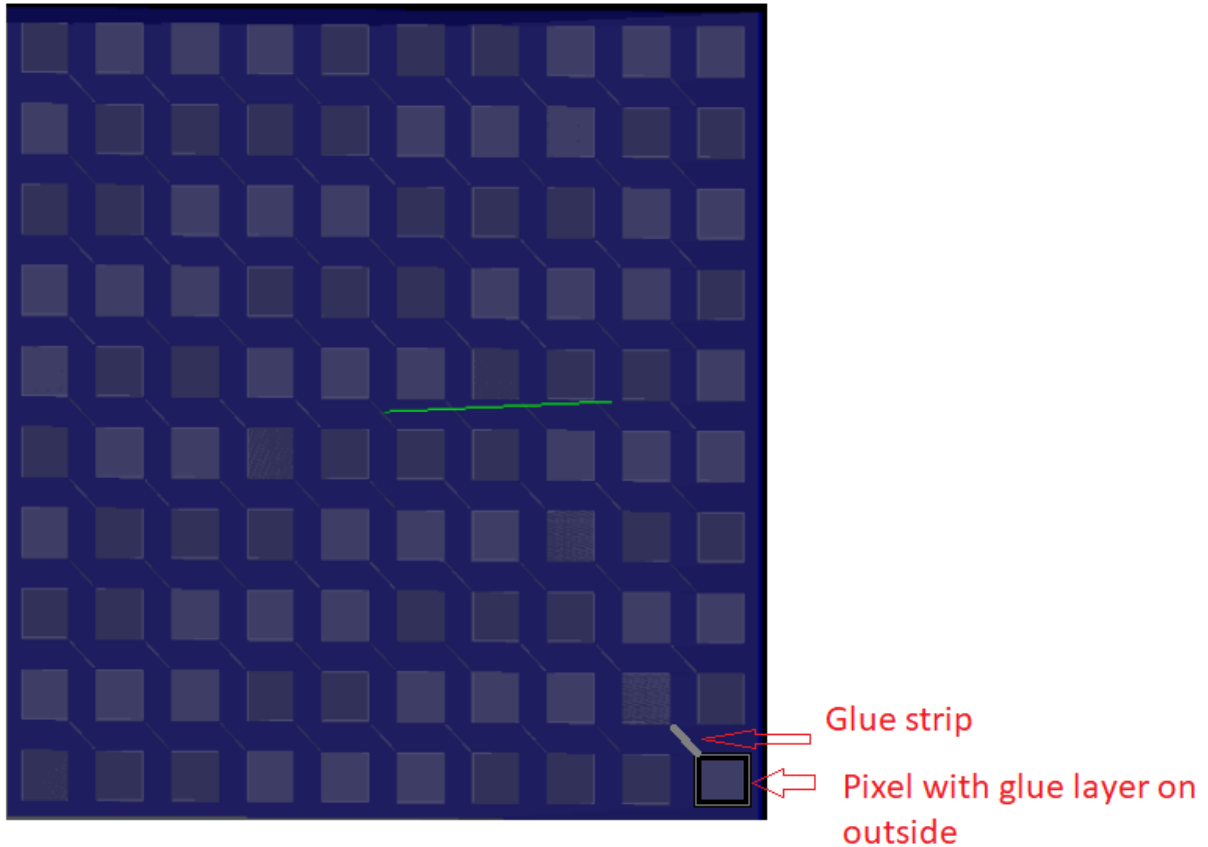
Figure 2.15 Close up of the new detector design for the optimization experiments. The glue was placed in the corner of the pixels since it was thought to be easier to build the detector this way.
