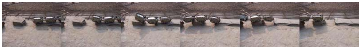
Figure 2-7: JL-1 in docked state overcoming the same trench
