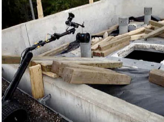
Figure 2-8: Large Talon robot unable to cross the gap and wall delivers a small Toughbot (seen in the gripper of Talon) into a roof opening.
