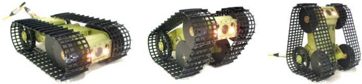
Figure 2-5: VGTV-Xtreme in its three main positions. In the lowest position for flat surfaces (left), middle position for climbing (center), top position for looking over obstacles (right).
