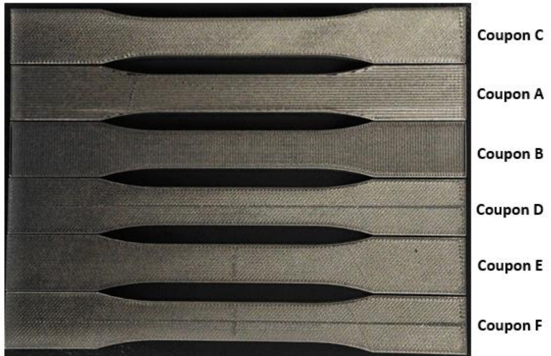
Figure 23 shows one coupon printed per each configuration (Coupons A-F) using Prusa i3 Mk2S.
