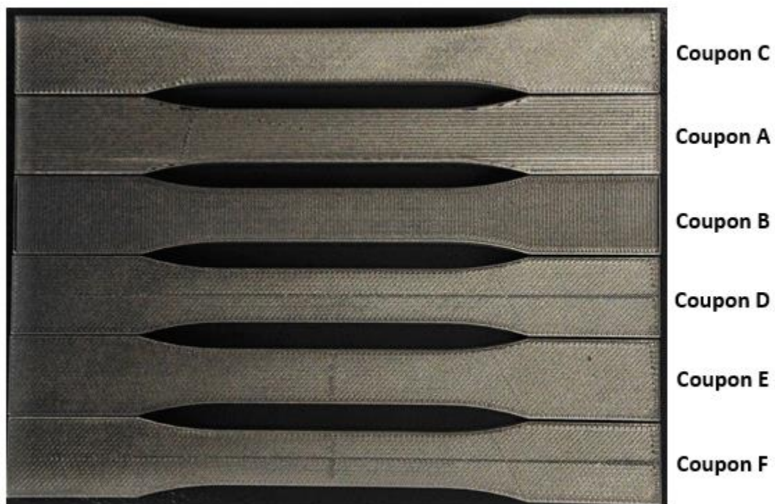
Figure 23 shows one coupon printed per each configuration (Coupons A-F) using Prusa i3 Mk2S.
