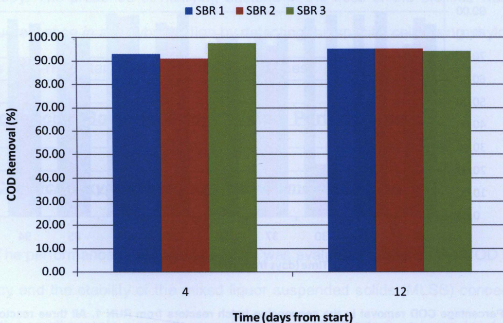
Figure 4.3 Percentage COD removal in the sequencing batch reactors from RUN 3. Reactor 1 and 2 were fed a synthetic wastewater with COD:N:P ratio of 100:5:1 and reactor 3 was given a P-limited feed of COD:N:P ratio of 100:5:0.33
