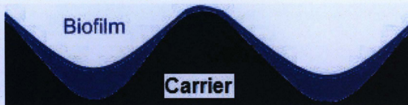
Figure 4.30 Diagram of biofilm growing in the grooves on the outer surface of the carrier material.
