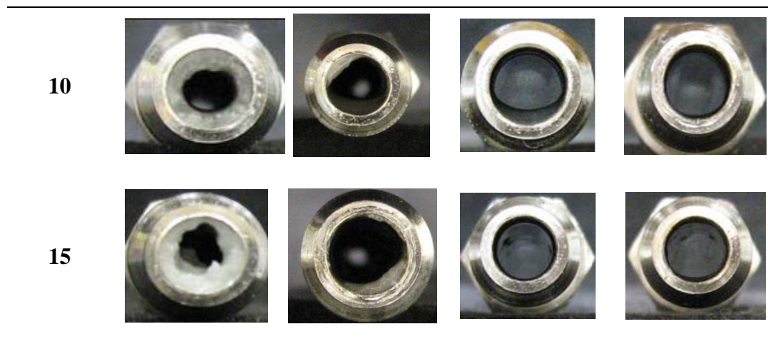
Figure 16: Loop section pictures at the end of the 30 hr flowloop runs at 25°C and 4°C.
