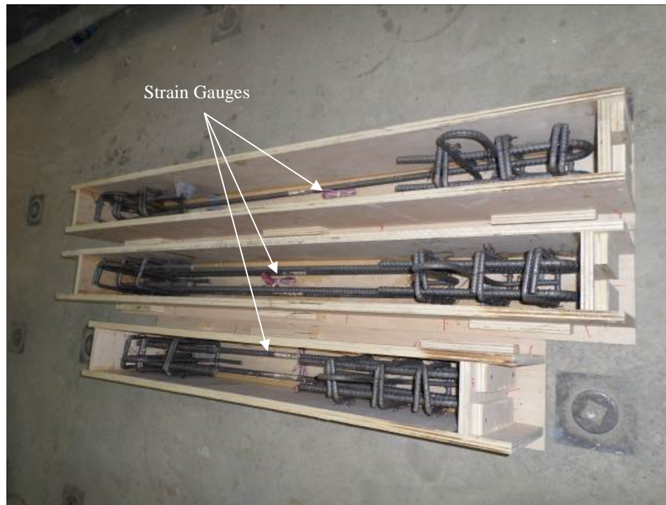
Figure 6.4: Strain measurements of longitudinal tensile reinforcements
