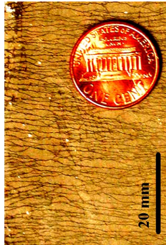
Figure 2.2: Crack formation in HPFRC (Li, 2003)
