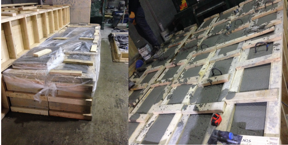
Figure 3.3.b – Manufacturing of HS-RC test beams - Casting of HS-RC beam specimens
