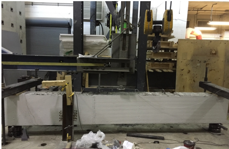
Figure 3.5.a – End supports arrangements of the beam specimen under testing
