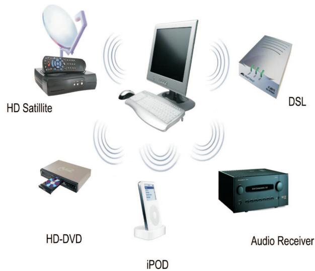
Figure 1.1: An example of an UWB wireless personal area network.
