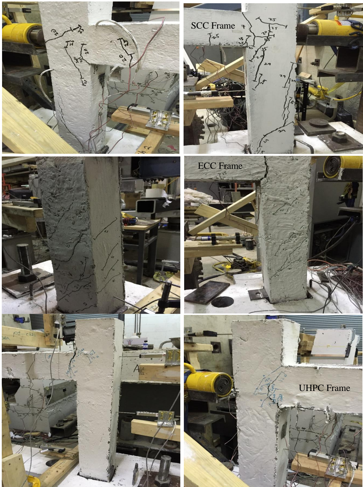
Fig. 4.10: Crack development and failure modes of shear-critical SCC/ECC/UHPC frames
