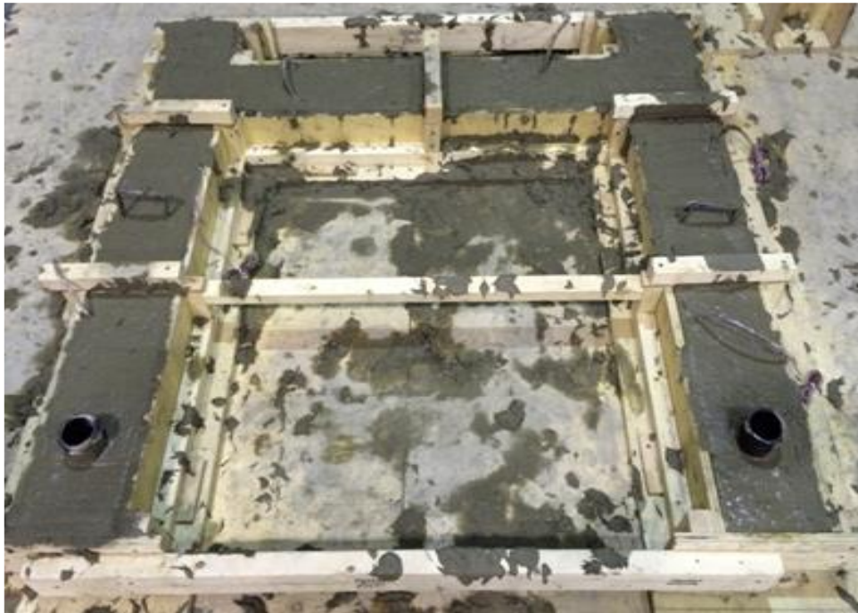
Fig. 3.8(a): Typical model frame and formwork after casting with control specimens
