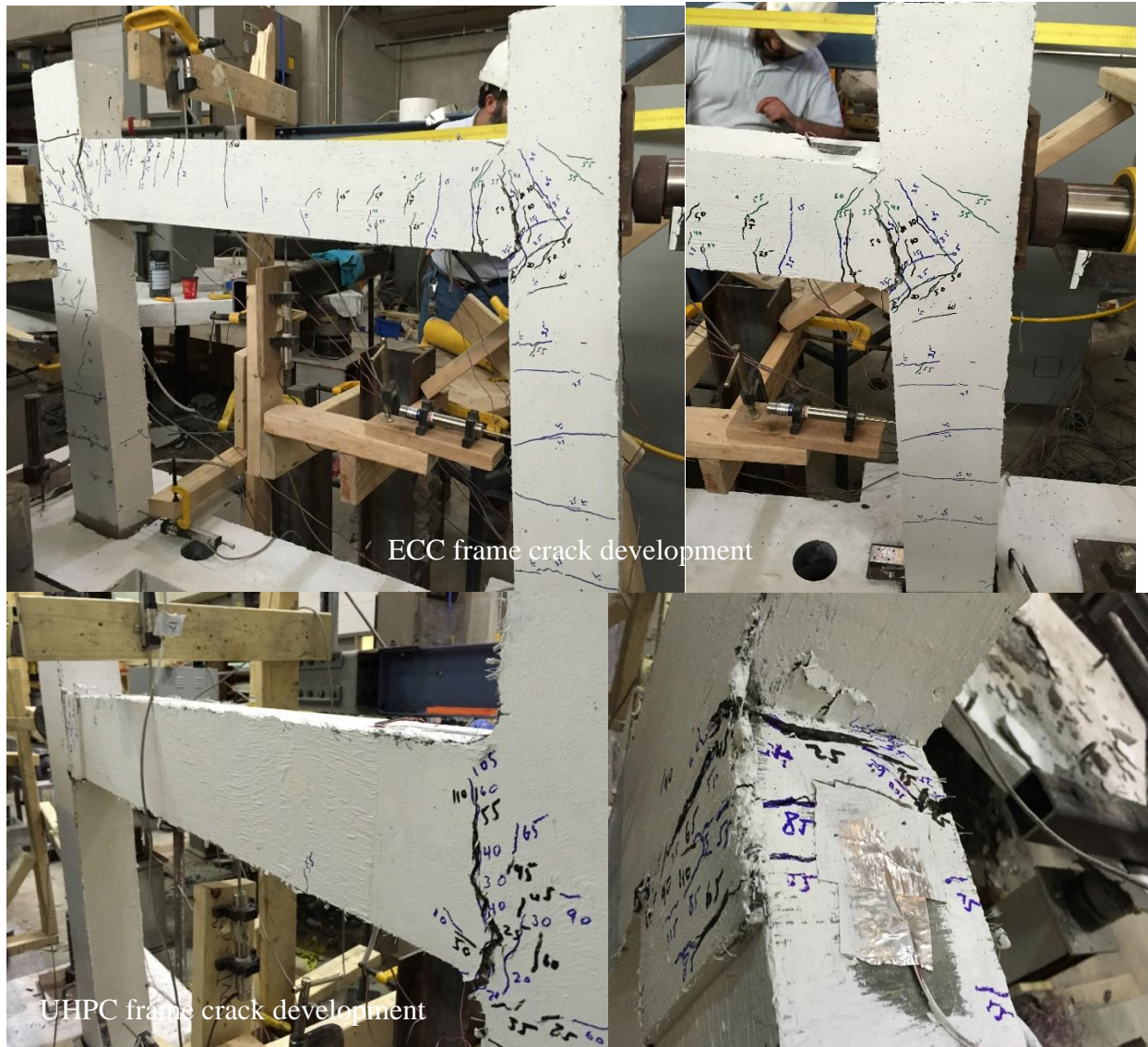
Figure 4.4(b): Crack development and failure modes of ECC/UHPC frames
