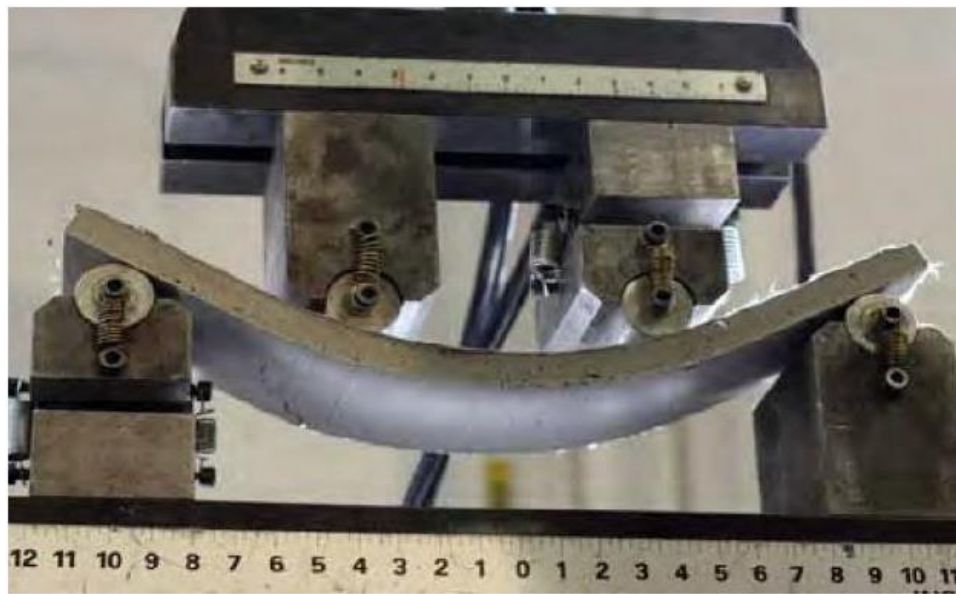
Fig. 2.2: Ductile response of ECC under flexural loading (Li 2011)
