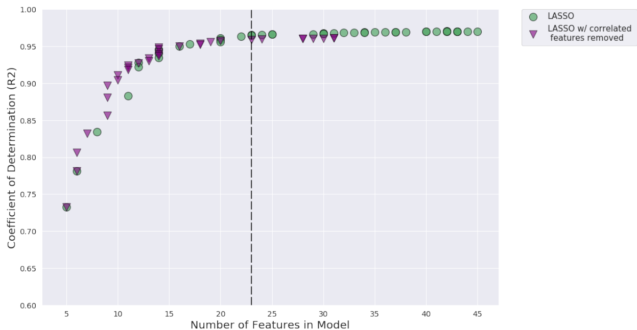
Figure 41 – Model coefficient of determination as the number of features in each the LASSO with correlated features (green circle) and LASSO with correlated combined features removed (purple triangle) models change. The selected number of features for both methods is shown by the dashed line.
