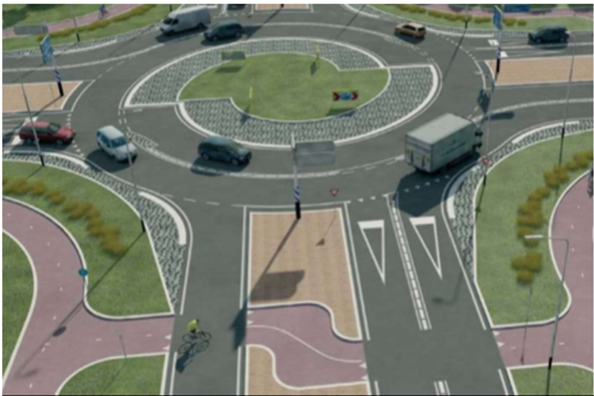
Figure 10: Turbo roundabout and its geometric features(Murphy & Manager, 2015)
