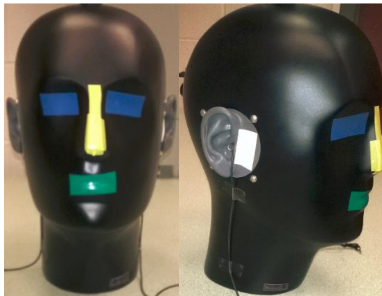
Fig. 4.2 Acoustic Dummy with facial feature stickers.
