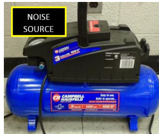
Fig. 3.26 Compressor used to generate experimental noise.
