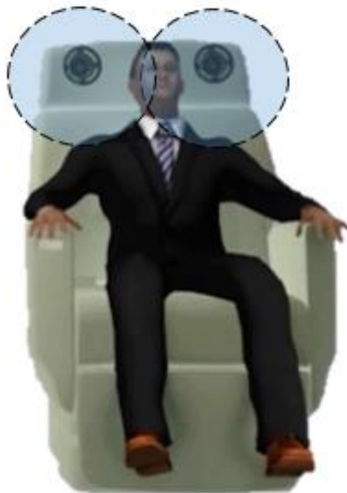
Fig. 3.1 Illustration of Zone of Quiet concept.
