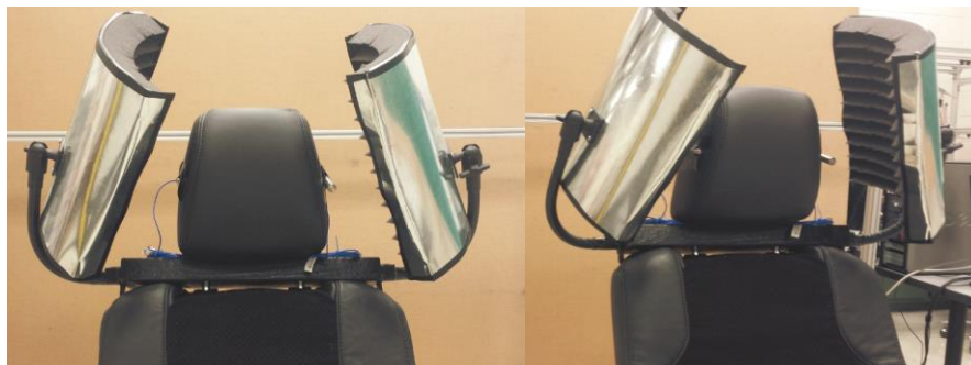
Fig. 3.28 Passive Noise Control setup with curved acoustic-grade foam wedges.
