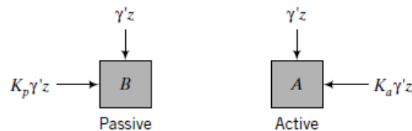
Figure 3: Principal Effective Stresses acting upon Soil Elements on Active and Passive Sides of a Retaining Wall
