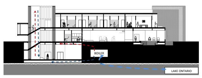
Figure 4.52. Water quenches Fire: Deep – Lake Geothermal Exchange, Hydronic Radiant Heating
