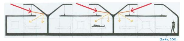
Figure 3.10. Section – Filtered Daylight
