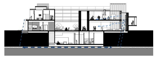
Figure 4.50. Water nourishes Wood: Rain Water Recovery, and Living Wall
