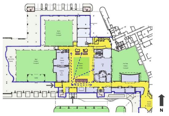
(Courtesy of Diamond + Schmitt Architects Inc.) Figure 3.33. Apotex Centre – Main Floor, Circulation and Orientation
