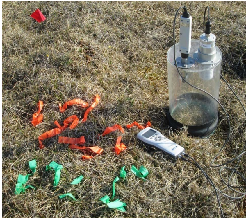
Figure 10: \text{CO}_2 flux static chamber light measurement and ion exchange resin strips in situ
