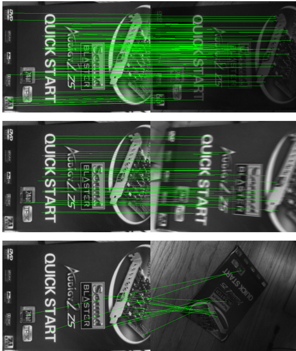
Figure 2.4: GPUSURF feature matching with illumination, motion blur, and combination changes.
