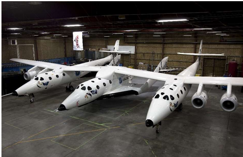
Figure 4 the Scaled Composites Space-Ship-Two (Central Fuselage) Resting under Its Mothership, White Knight Two, inside a Hangar in Mojave, Ca., USA
