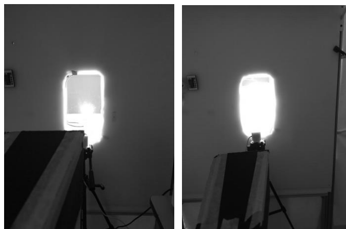
Figure 3.17 View from inside the mock up without optics enhancement (left) vs with optics enhancement (right)
