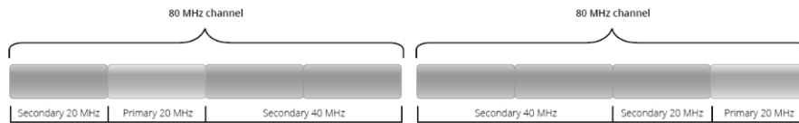
Figure 1.3: IEEE 802.11ac channelization for 80MHz band [2]
