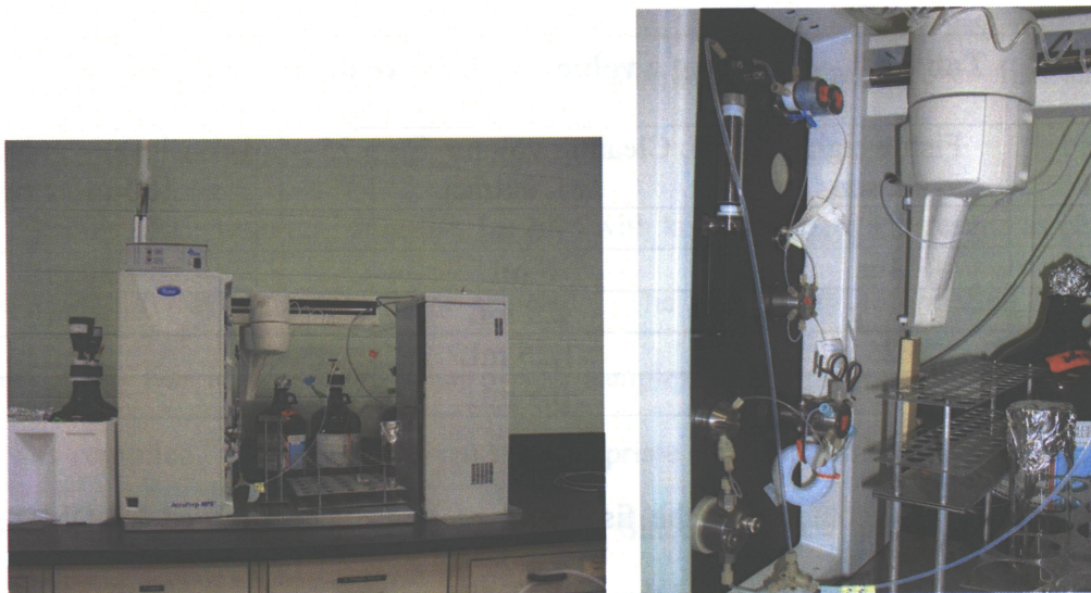
Figure 3.1 – GPC instrument (left) and close-up of automated sampler arm of GPC (right).
