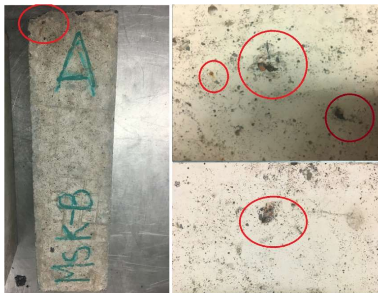
Figure 6.32. Deterioration and rust in concrete prisms with MSK
