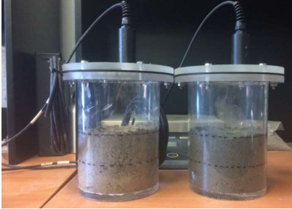
Figure 3.2. OCT set-up showing sealed plexiglass cells with 100-mm crushed aggregates
