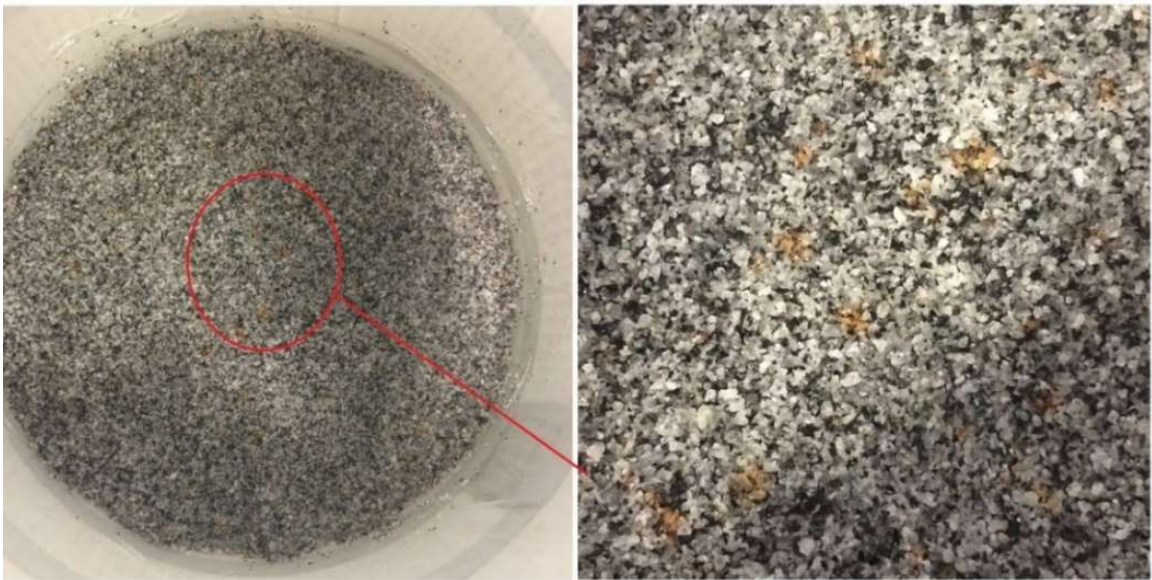
Figure 4.2. Rust in aggregate crushed by disk pulverizer with iron plates to a size of (600 \mu\text{m} to 300 \mu\text{m} )
