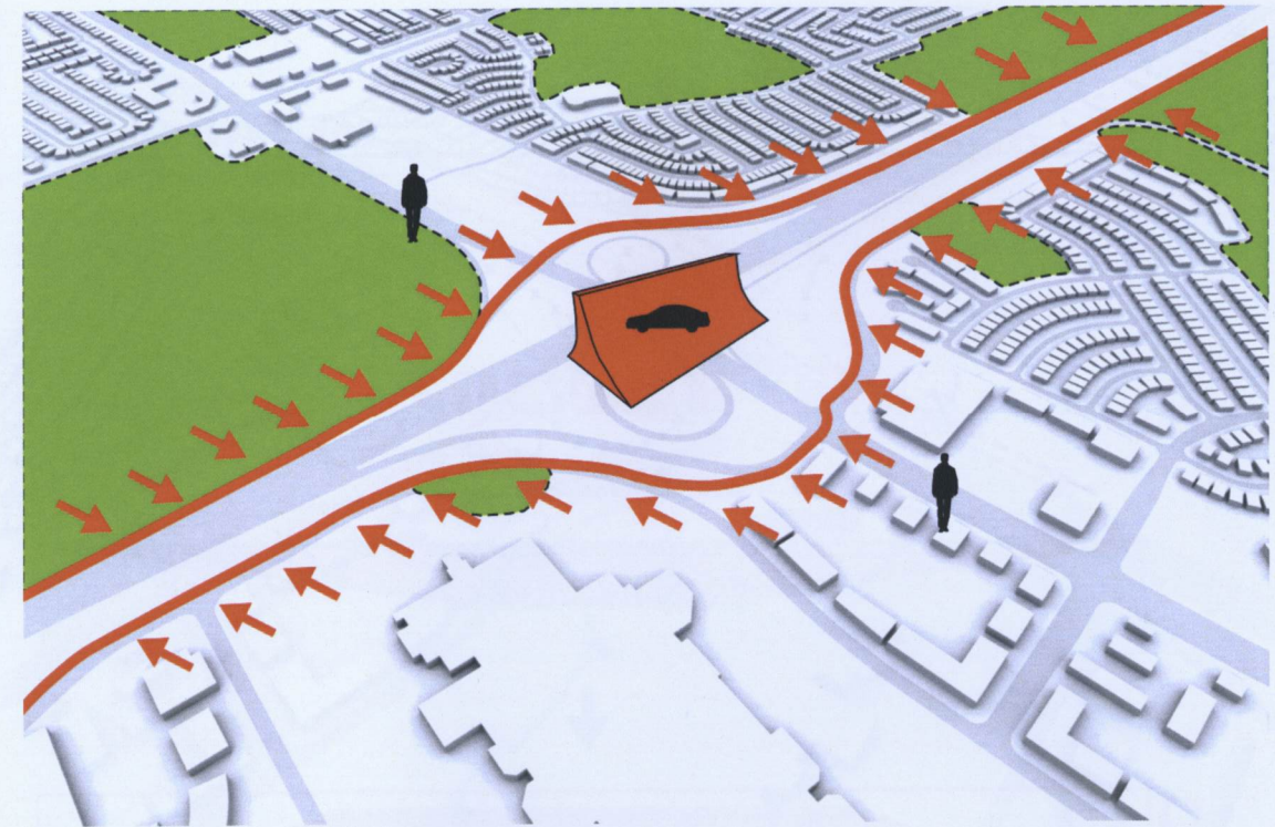
Figure 6-16. Diagram illustrating the barrier that the interchange imposes on pedestrians and the surrounding neighbourhoods.
