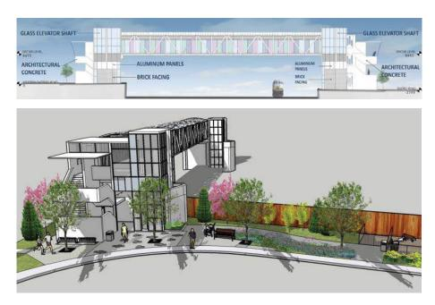
Figure 5.35: Proposed pedestrian bridge connecting Douro St and Western Battery Rd
