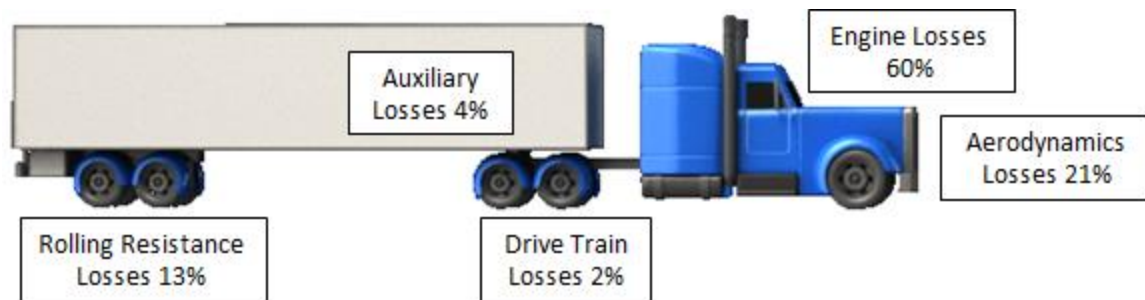
Figure 3: Tractor trailer energy losses (USDOE)
