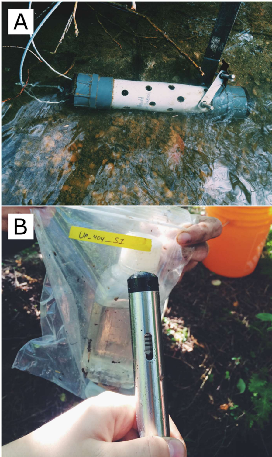
Figure 10: A) Custom made levellogger casing anchored in position and B) a Solinst LTC Levellogger from the UP_404_S1 site in East Holland.
