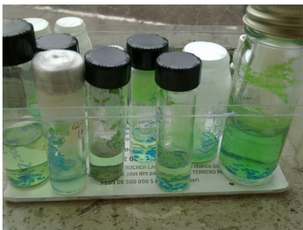
Figure 16: Blue and green crystals appearing in the acetonitrile solvent. Nitrate sources for the three different bottles at the front of picture: (a): \text{AgNO}_3 ; (b): \text{Ni}(\text{NO}_3)_2 \cdot 6\text{H}_2\text{O} ; (c): \text{NaNO}_3 .
