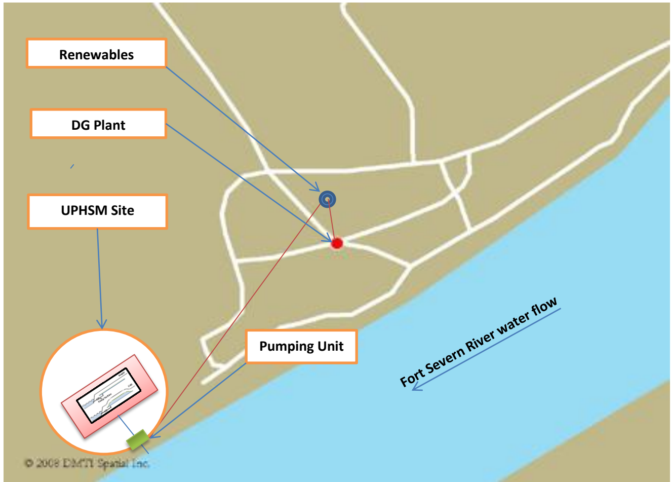
Figure 4-15 Schematic diagram of UPHSM System integrated with Renewables and DG Plant
