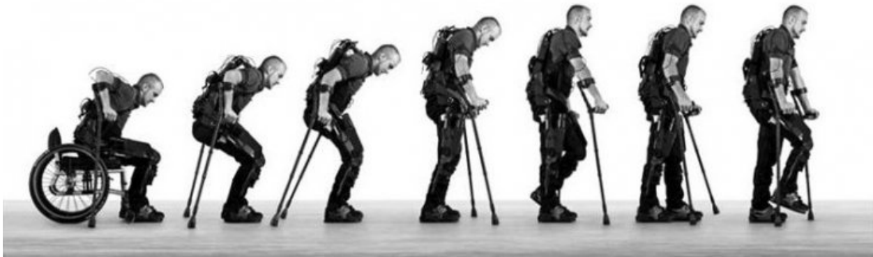
Figure 1.2: Sit to Stand and Stepping in a lower body exoskeleton (from Ekso Bionics and [25])
