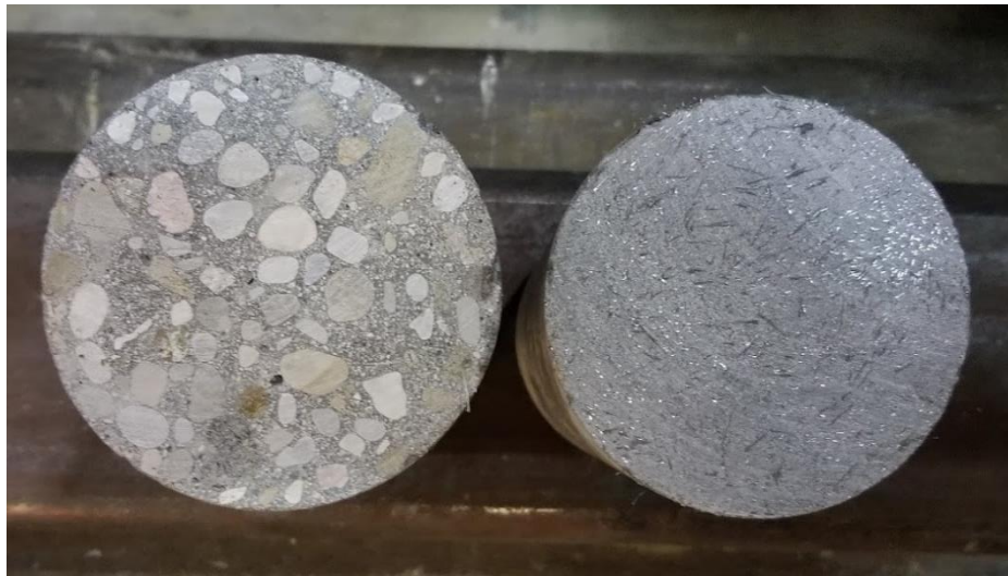
Figure 3-7: HSC (left) and UHPC (right) Samples Cut and Polished
