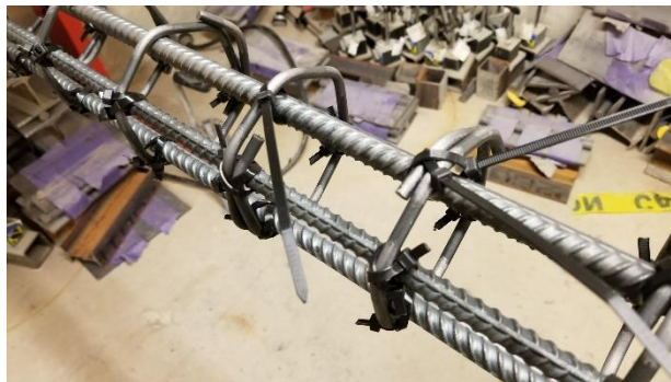
Figure 3-5: Close-up of Transverse Reinforcement Connection to Longitudinal Rebar
