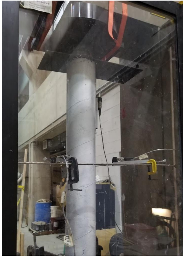
Figure 3-11: Position Transducer Placement During Compressive Testing
