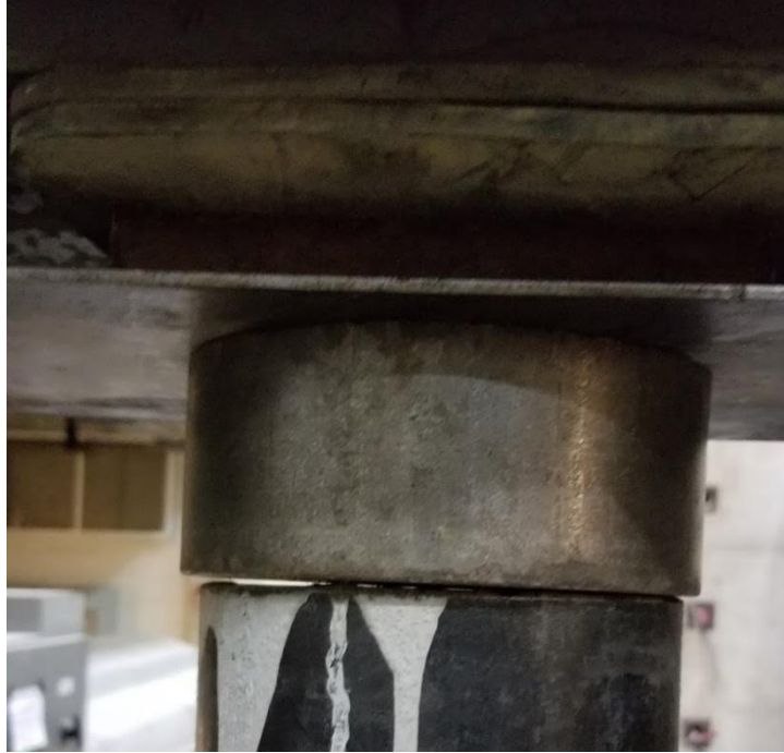
Figure 3-10: Top Portion of Loading Specimen with the Rubber Layer (top)
