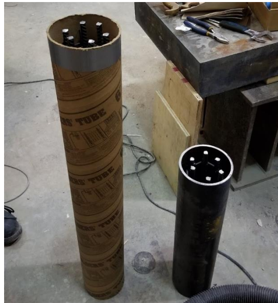
Figure 3-1: Unconfined (Left) and Confined (Right) Column Formwork
