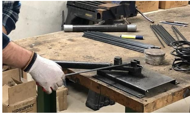
Figure 3-2: Bending the 6-M Rebar for Transverse Reinforcement
