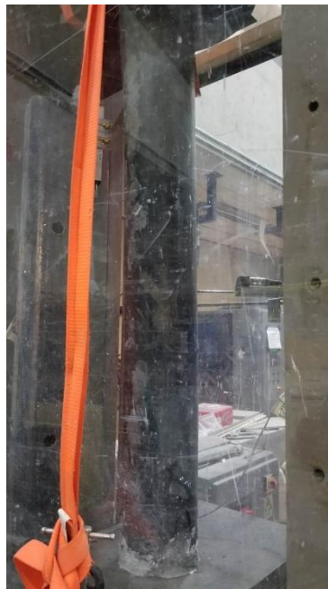
Figure 3-9: Compressive Testing Set-up with Plexiglass Protection
