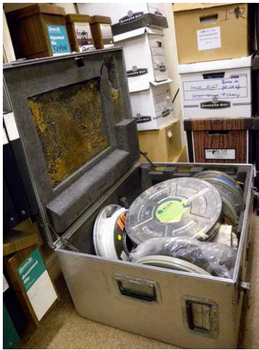
Fig. 20 - Metal trunk with poorly ventilated acetate reel film suffering from vinegar syndrome. Photograph by author. Courtesy of the Royal Ontario Museum.
