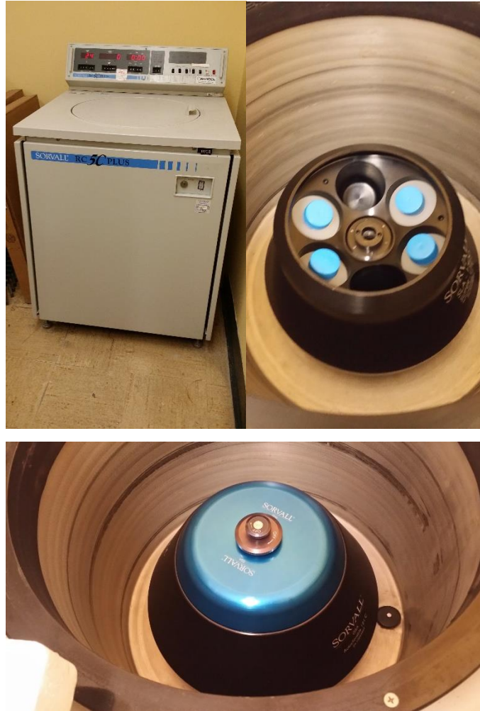
Figure 3.5: Centrifuge machine (left), falcon tubes kept in the rotor inside the centrifuge machine for centrifuging (right), rotor with cover ready for centrifuging (bottom)
