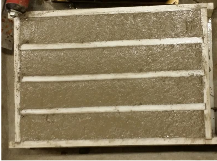
Figure 3.11: Mortar prisms with moulds
