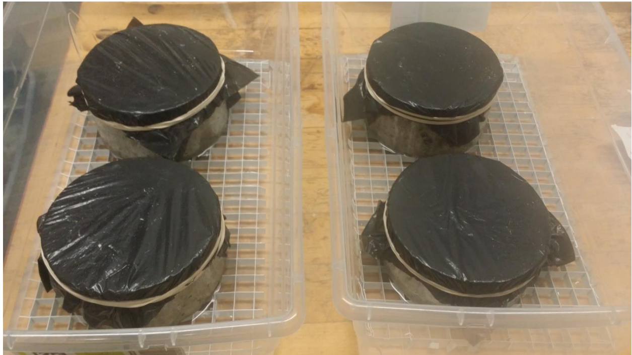
Figure 3.15: Test set-up for sorptivity test
