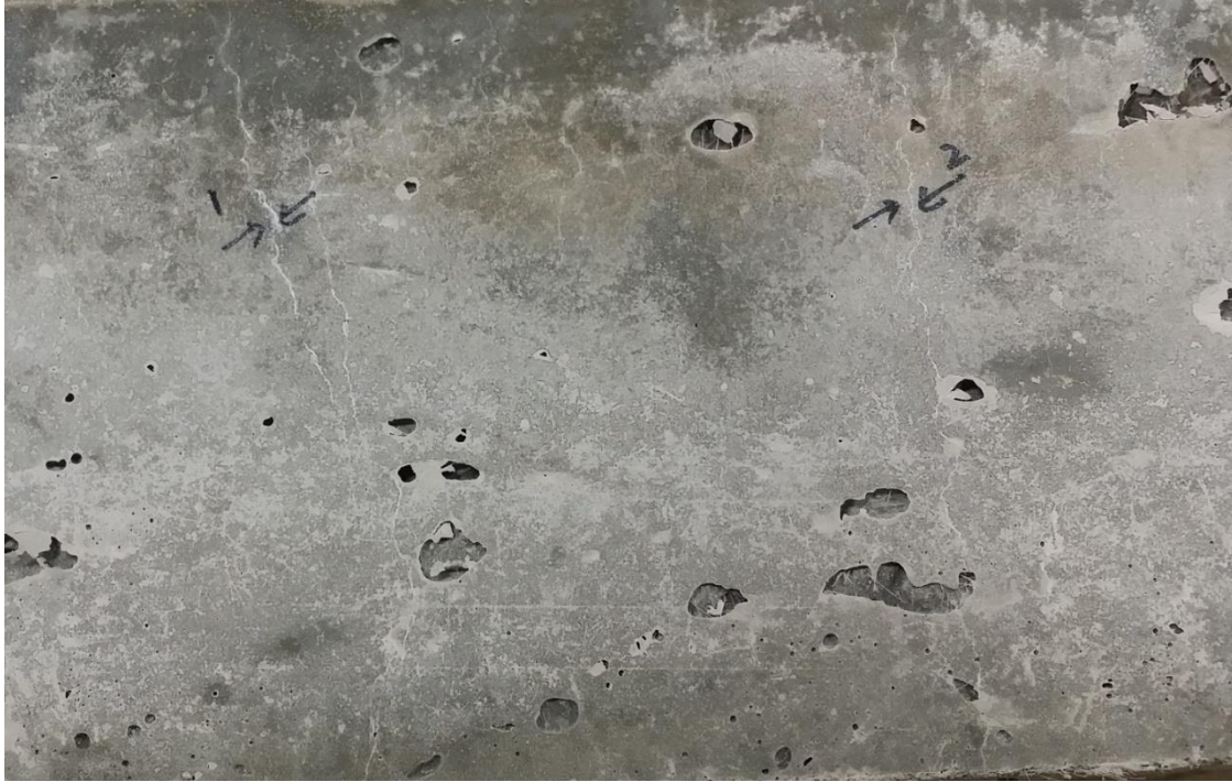
Figure 4.79: Healed specimens with Bacillus subtilis immobilised into zeolite
