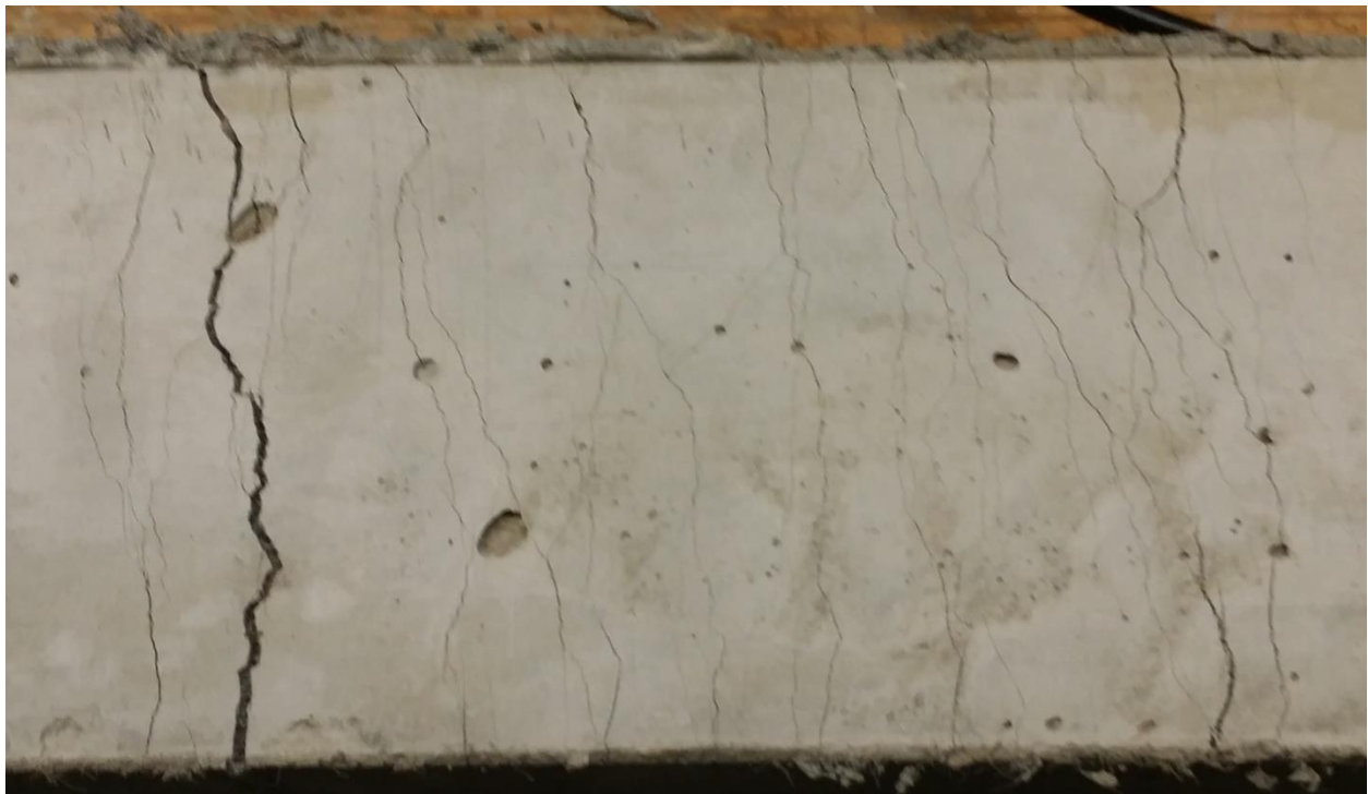
Figure 3.20: Typical failed sample of bacteria based ECC with macro crack and multiple micro cracks
