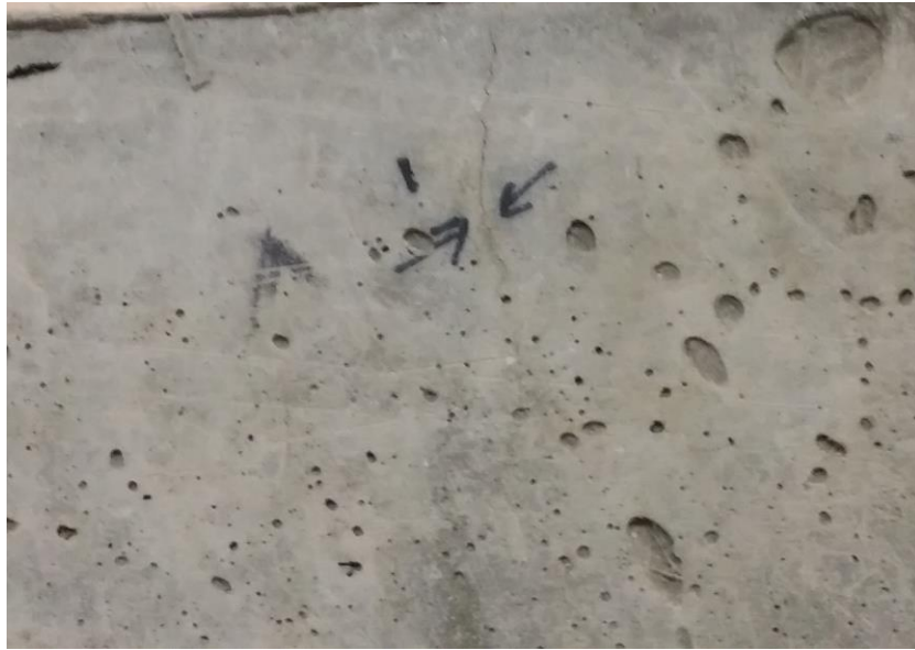
Figure 4.76: Control specimen with no visible crack healing
