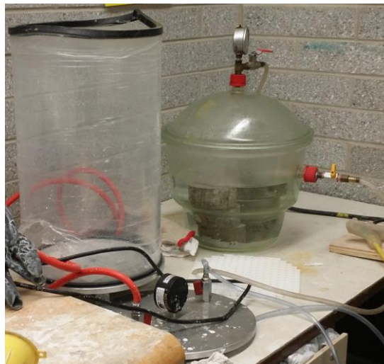
Figure 3.16: Specimen submerged in dessicators bowl
