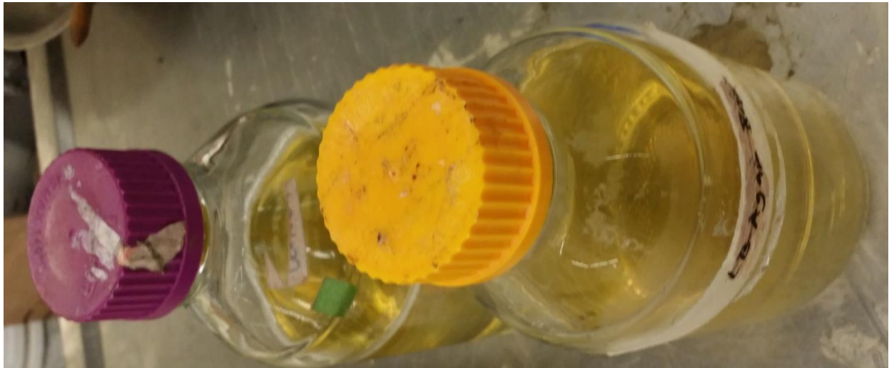
Figure 3.8: Dissolved nutrient solution used as part of mixing water
