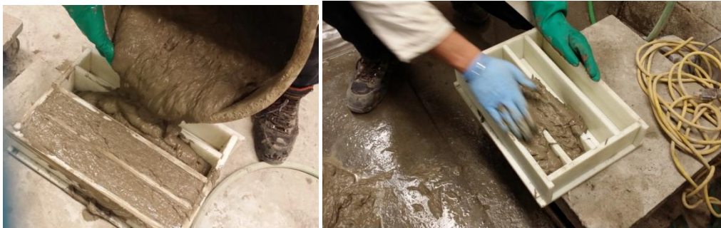
Figure 3.19: ECC mixture pouring in the prism mould
