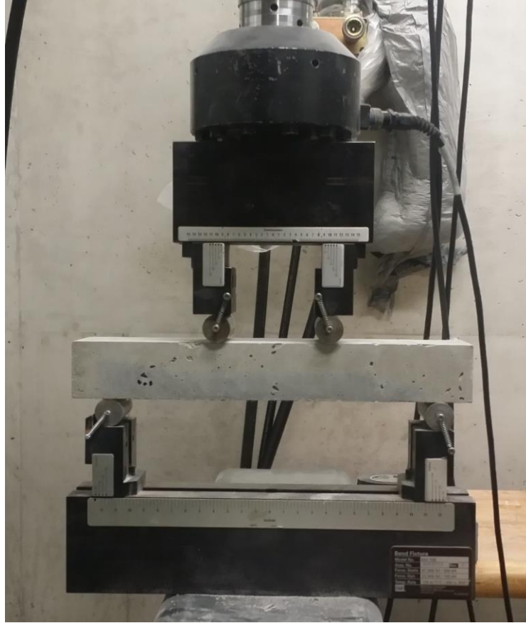
Figure 3.12: Test set up for four point bending test
