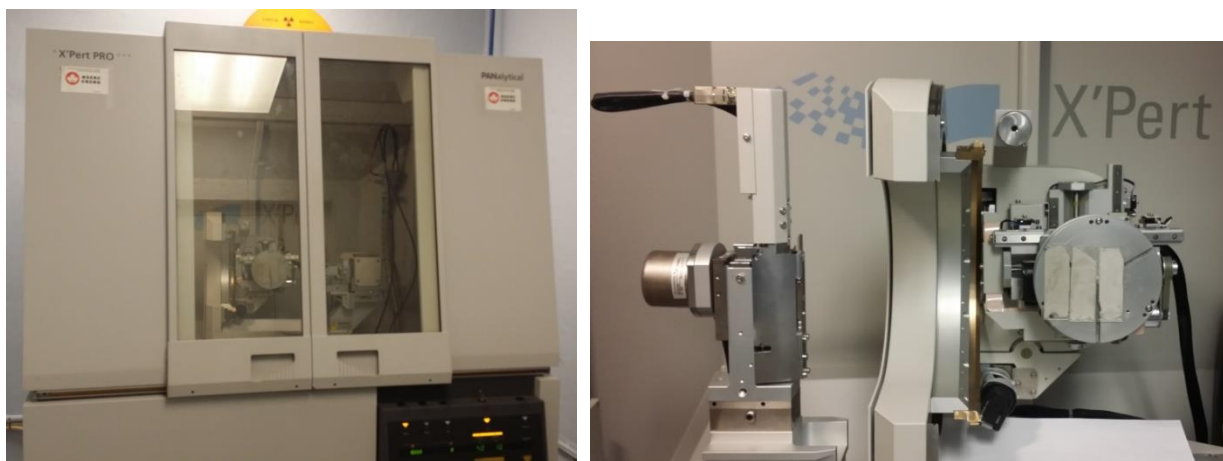
Figure 3.18: X Pert PRO apparatus (left), samples mounted on the X Pert PRO apparatus
