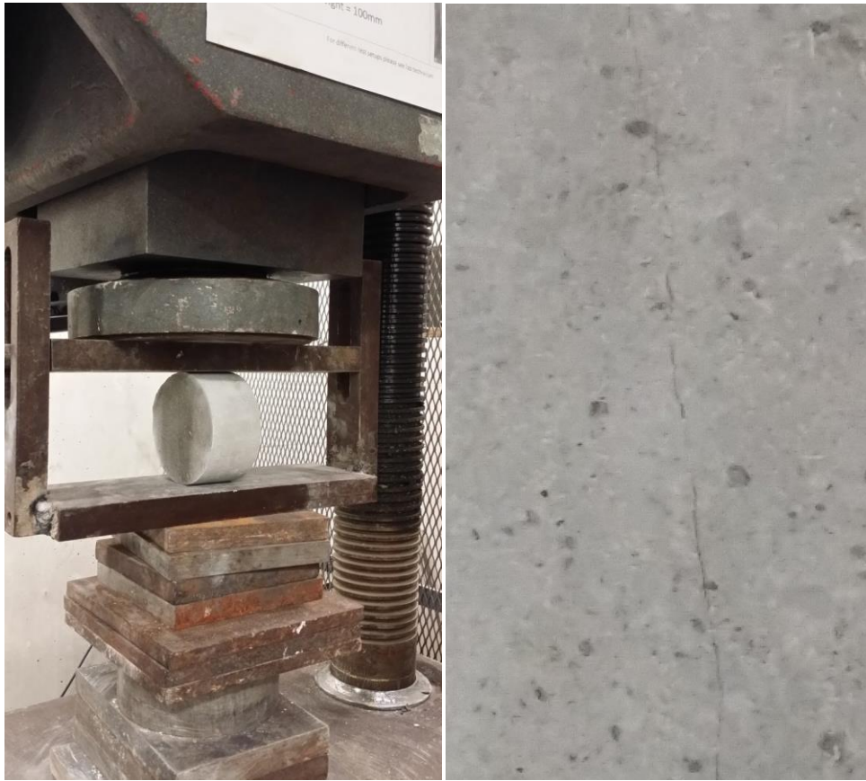
Figure 3.14: Tensile splitting test set up to induce cracks (left) and the induced crack (right)
