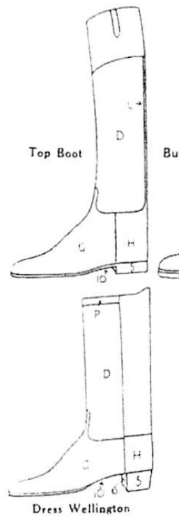
Figure 10. Construction differences between the Top boot and Wellington boot. 10
