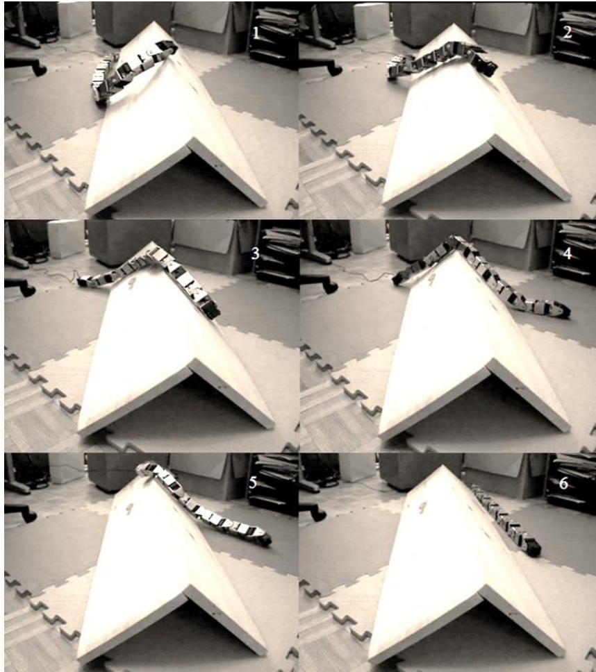
Figure 4.2.4: Striker overcoming OMT using the SG2 gait.
