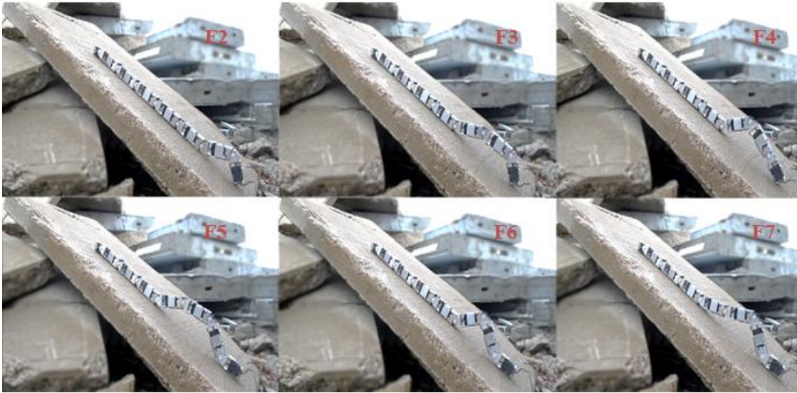
Figure 4.3.4: Using the Hillz gait, Striker climbed an inclined concrete slab in a real settings.
