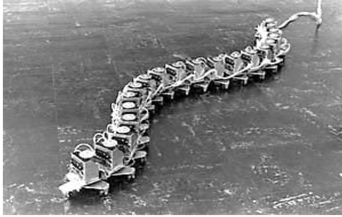
Figure 2.6.3B: Active cord mechanisms III using Serpenoid Curve
