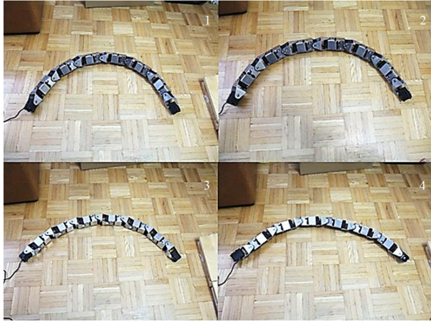
Figure 4.2.1B: the lateral rolling gait pushed Striker on its side (upward) by contracting and expanding the arc.
