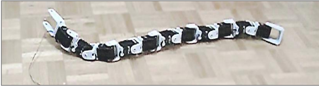
Figure 3.2A: Prototype S1 with links connected with plastic brackets.
