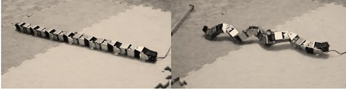
Figure 4.2.3: SG1 gait containing 2 Frames, Frame 1 and Frame 2 respectively.
