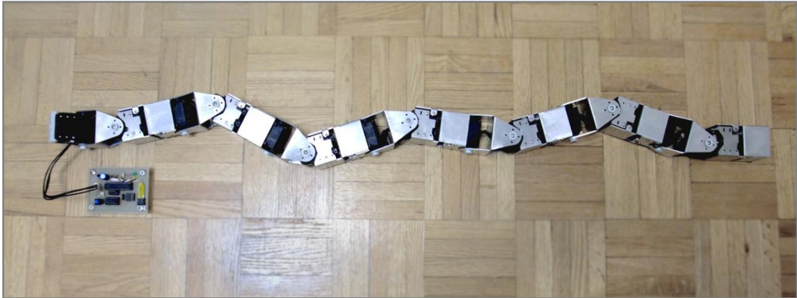
Figure 3.3: Striker; composed of one NSR microcontroller and 7 modular segments.
