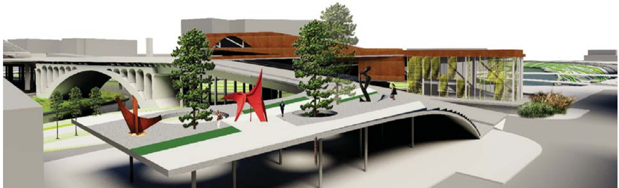
Fig 171. Spaces such as the outdoor exhibit over farmers market is created by extending the bridge deck. Pine trees that can grow between 15-30 meters tall provide an opportunity as a shading element for the exhibit space.
