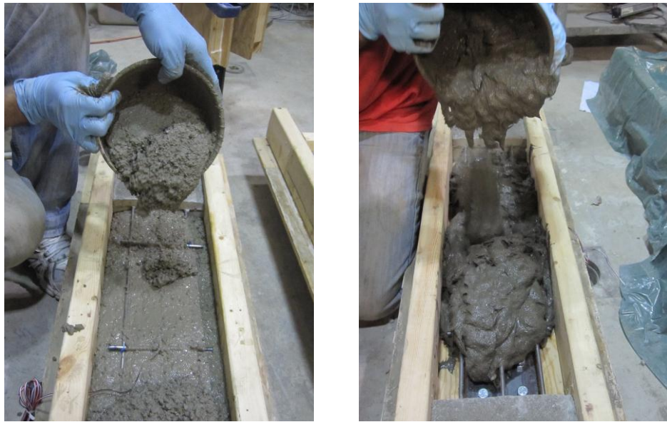
Figure 3.7 SCC to the left and ECC to the right, excellent workability eliminating the need of vibration
