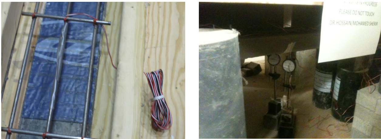
Figure 3.10 Instrumentation and measuring system for long-term creep test
