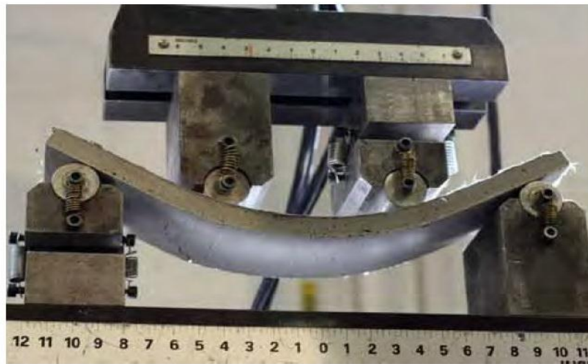
Figure 2.2 Extreme flexing capabilities of ECC under a large bending load (Li, 2011)
