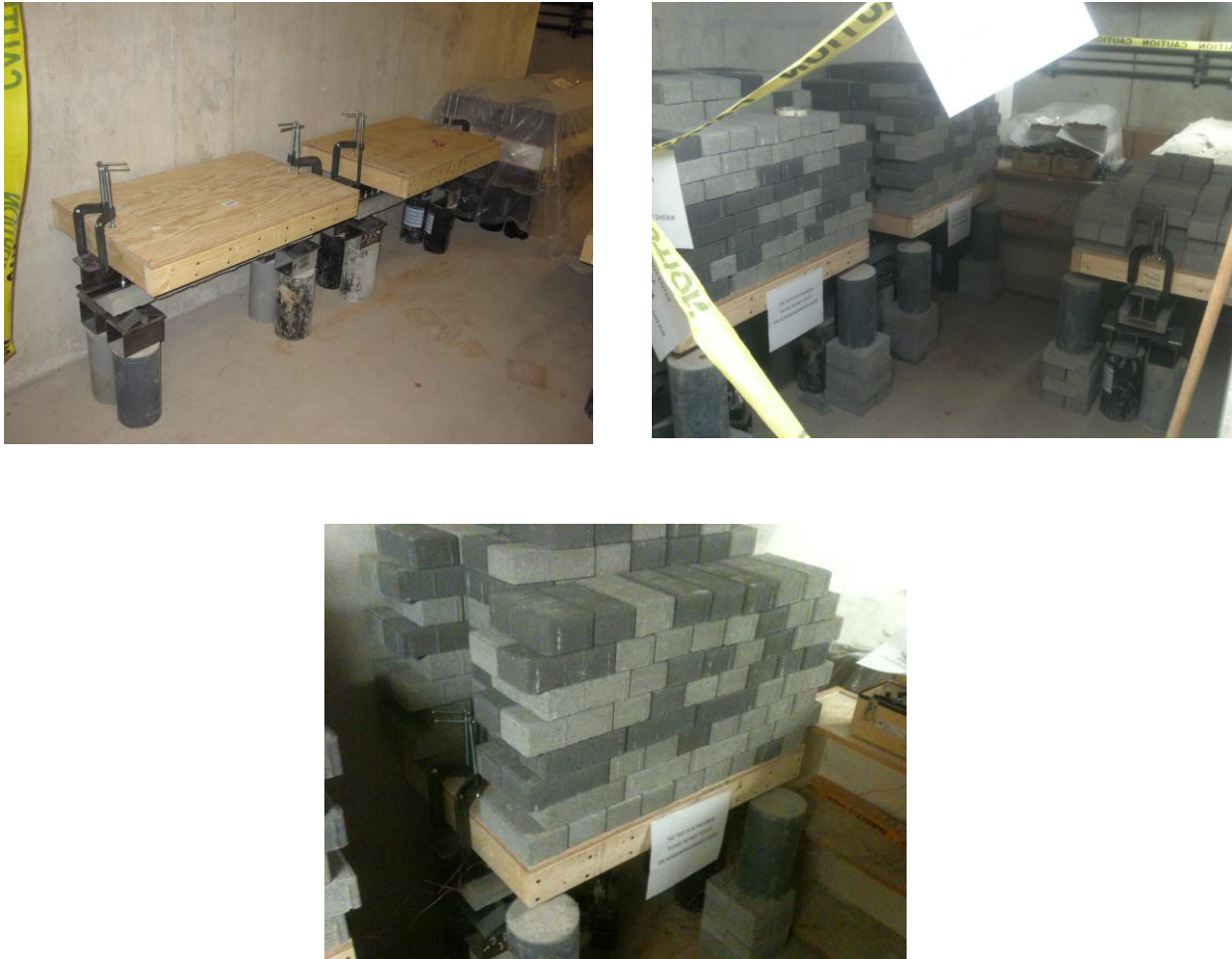
Figure 3.9 Test setup of long-term creep test
