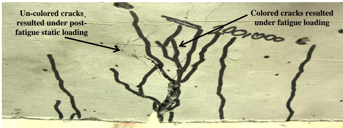
Figure 4.19 Multiple Cracking under Flexural Fatigue Loading
