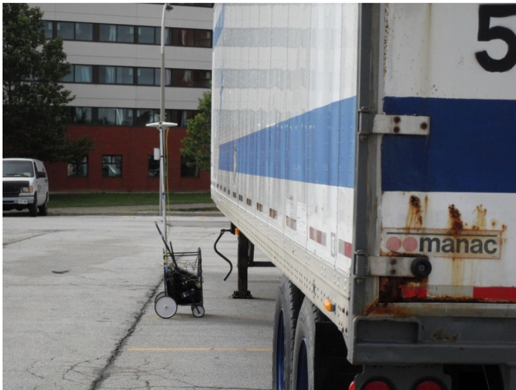
Figure 5.9 Kinematic data collection cart with the metallic structure for the KJU27 session
