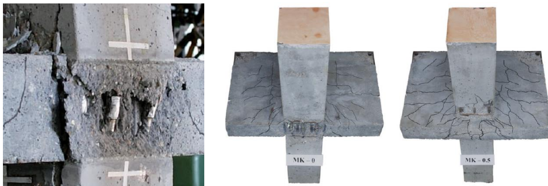
Figure 7-3 - Spalling of the concrete as a result of the non-existent overhang [1]
