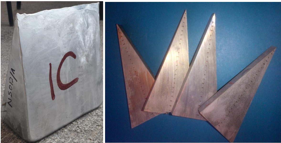
Fig.3.5. Wedge casting and slices (base 60x10 mm and height 120 mm) used for ageing experiment and hardness measurements.
