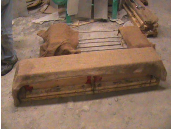
Figure 3.18: Wet burlap placed on Ryerson Concrete specimens following casting.
