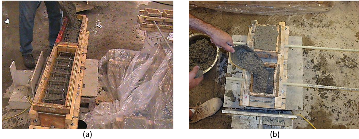
Figure 3.9: Bond test specimen casing with HP-S10 Concrete: (a) Beam test specimen; (b) pullout test specimen.
