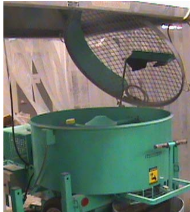
Figure 3.11: Mortarman® 750 MBP mixer used to batch Ductal®.
