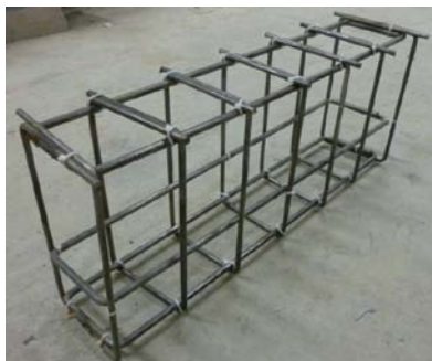
Figure 3.5: Reinforcement cage for Type B specimen.
