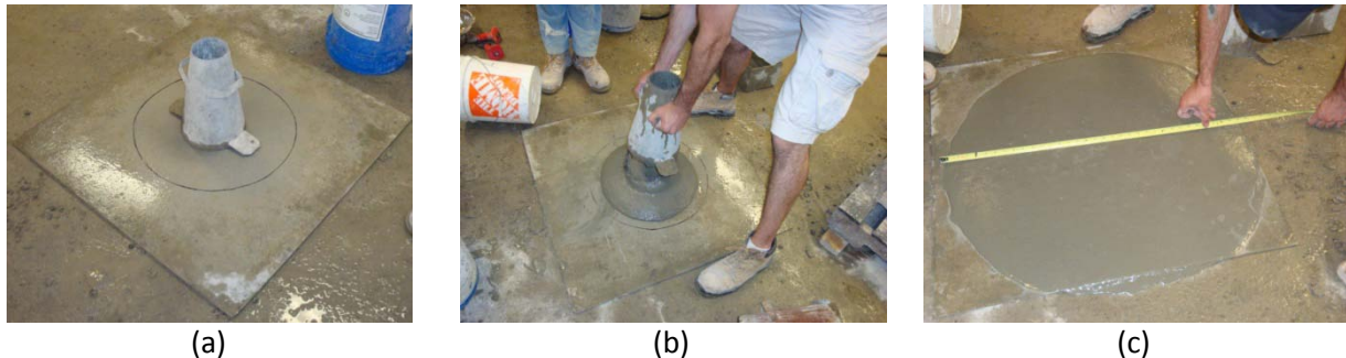
Figure B.2: Slump-flow and T_{500} test for Ryerson Concrete: (a) Slump cone and base plate; (b) lifting of the slump cone allowing concrete to flow; (c) measurement of the largest diameter of spread.
