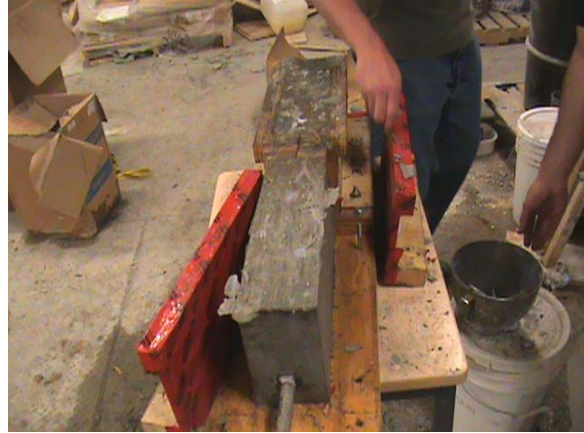
Figure 3.14: Demoulding of beam specimen.
