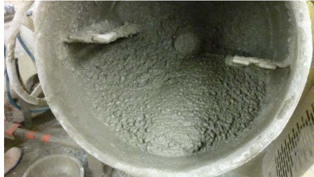
Figure 3.8: HP-S10 Concrete after mixing.
