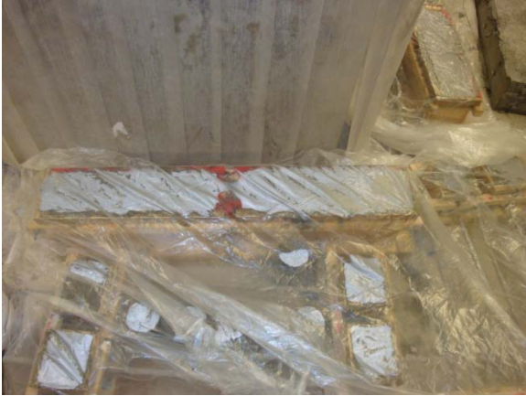
Figure 3.13: Sealed Ductal® specimens after casting.
