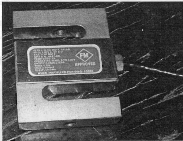
Fig. 6- Load cell was connected to a computer to register changes in force
