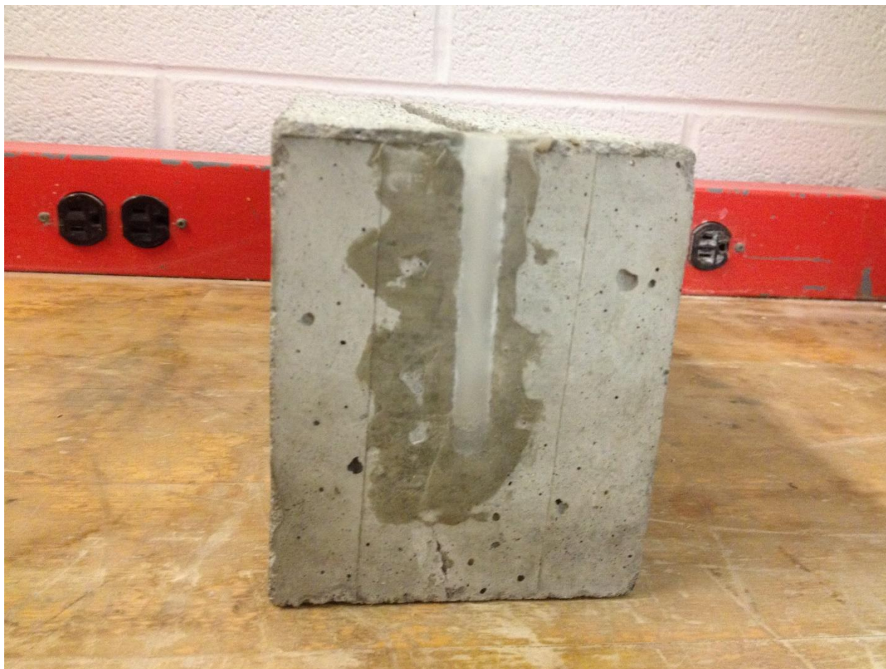
Figure 3-2 A rectangular slab with a sealed joint to prevent leaking of salt solution.
