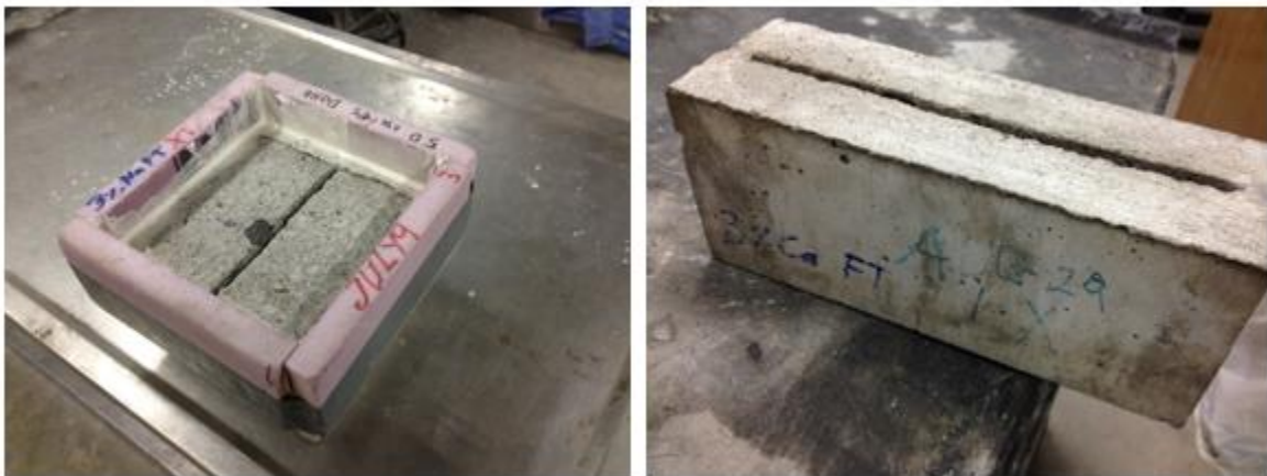
Figure 3-1 The two types of slabs used in the experiment: square slabs, 200 mm x 200 mm 120 mm (left) and rectangular slabs, 300 mm x 100 mm x 120 mm (right).
