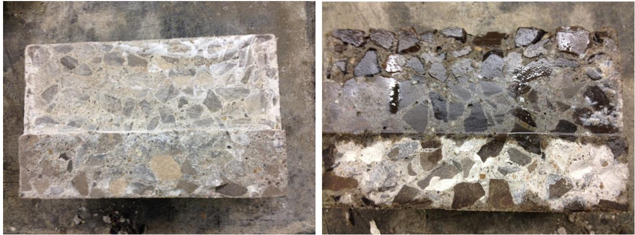
Figure 4-14 A view inside the joint (after loading) of the 10% NaCl FTW ( \text{H}_2\text{O} ) sample (left) and the 10% \text{CaCl}_2 FTW sample (right), both from the 45 MPa mix.
