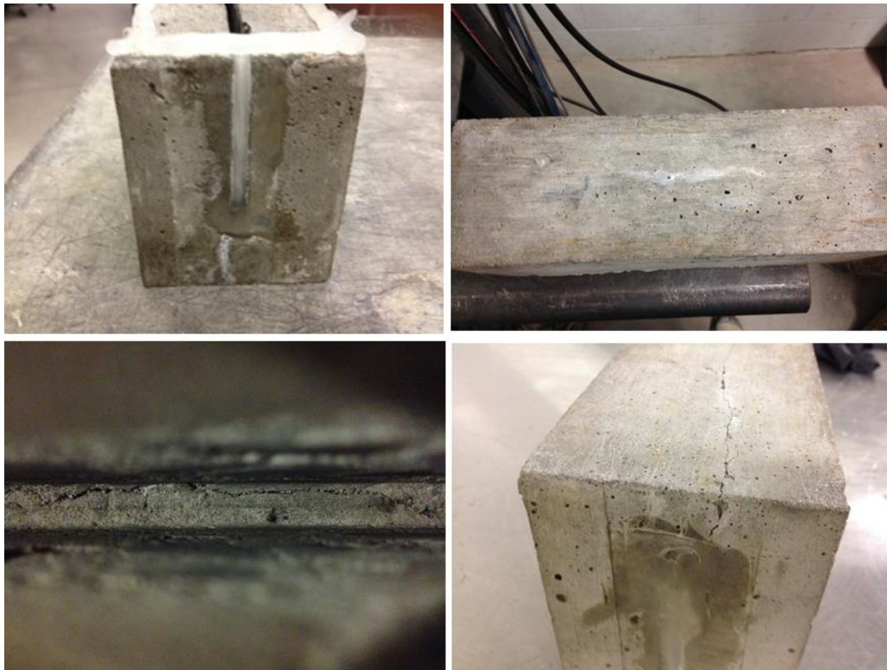
Figure 4-13 Cracks in and around the joint of slabs exposed to FT before loading. A crack and efflorescence below the joint of a 3% \text{CaCl}_2 FT sample (top left), some efflorescence and a thin crack on the bottom surface of a 3% \text{MgCl}_2 FT sample (top right), cracks inside the joint of a 3% \text{CaCl}_2 sample (bottom left), and a crack visible on the bottom surface of a slab connecting to the saw cut of a 3% \text{CaCl}_2 sample (bottom right).
