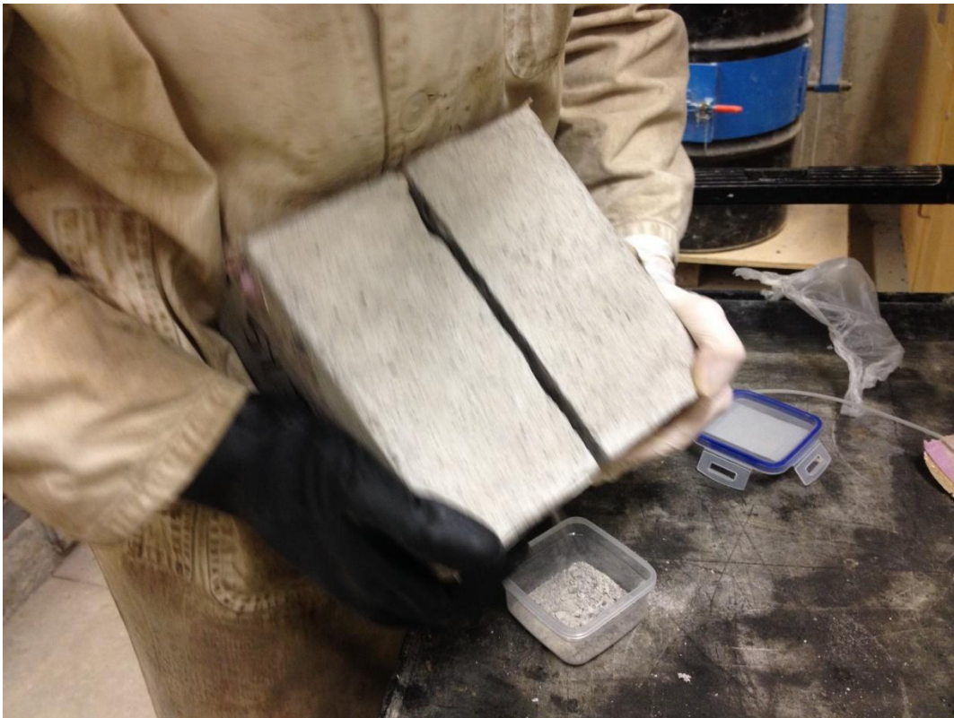
Figure 3-3 Removing material from inside the joint of a concrete slab and collecting it inside a container.
