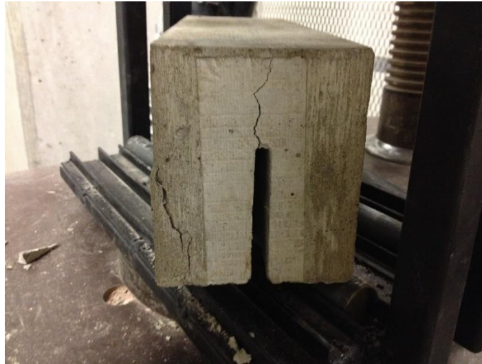
Figure 4-12 Control slab tested to ultimate failure, which had experienced some cracking above the roller support (left side of the image).
