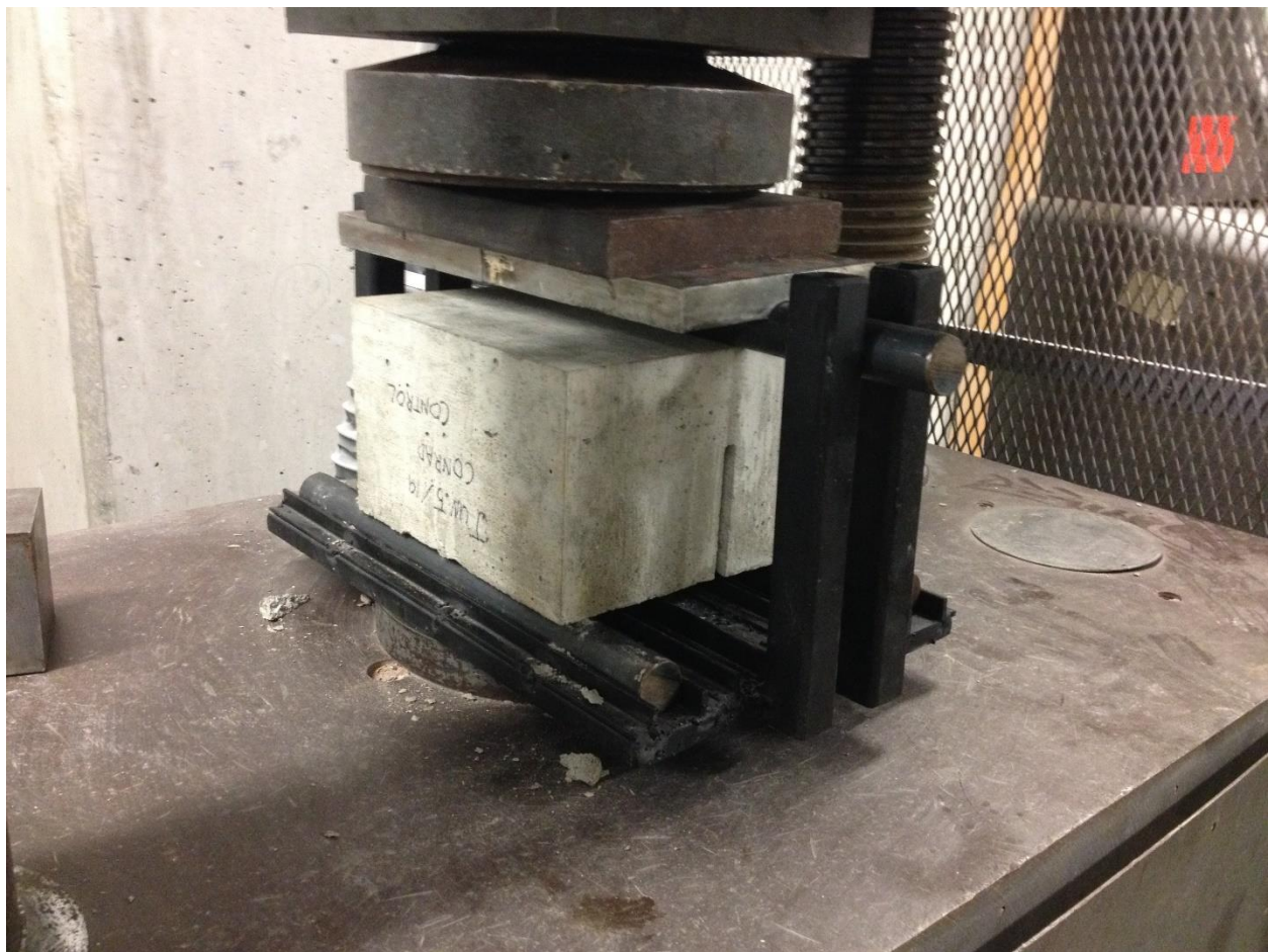
Figure 3-4 Square slab in the designed loading setup with adjustable rollers to load both the square and the rectangular slabs.
