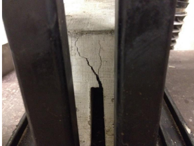
Figure 4-10 Control slab tested to ultimate failure with rollers, in which the crack that had formed was not confined to the section immediately above the saw cut.
