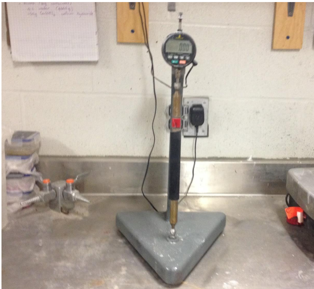
Figure 3-6 The Humboldt Length Comparator H-3250D with a comparator rod in place, used for measuring length changes of prisms.
