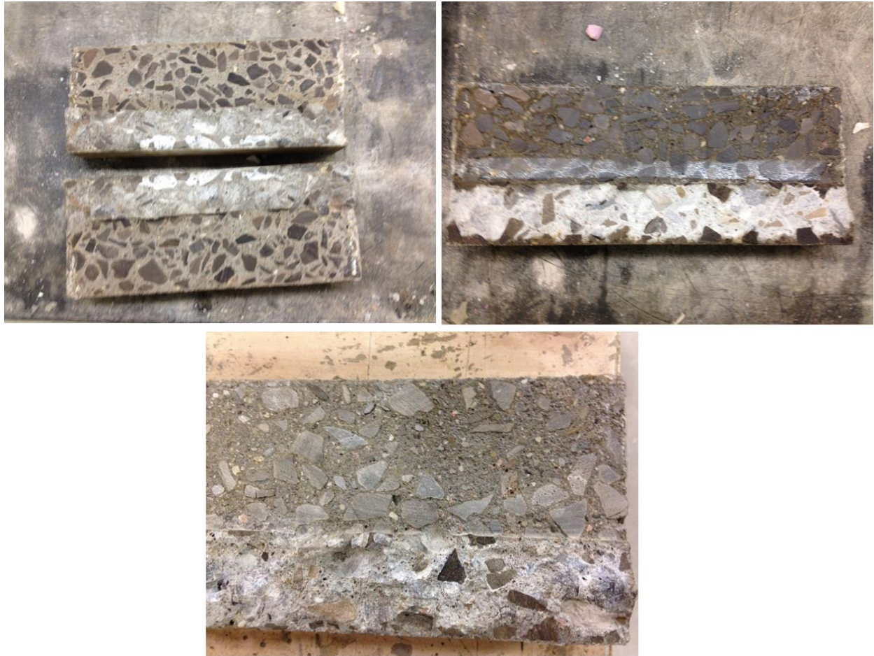
Figure 4-15 Inside the joints of different samples after loading: 15% NaCl W (top left), 15% MgCl 2 W (top right), and 3% MgCl 2 FT (bottom).
