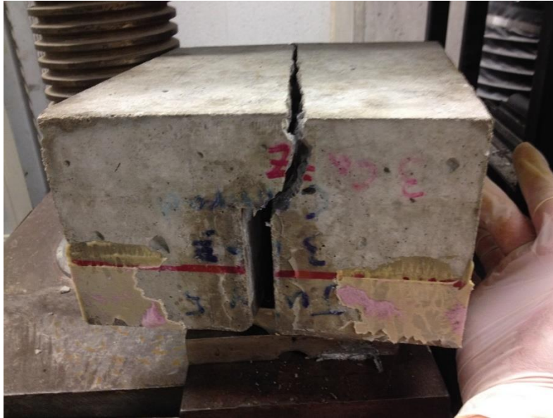
Figure 4-11 10% CaCl 2 FT sample with the crack extending up and away from the joint rather than staying confined within the area directly above the saw cut.
