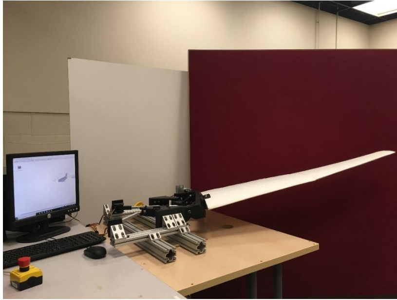
Figure 5-22: Prototype test setup with Winglet at 10°
