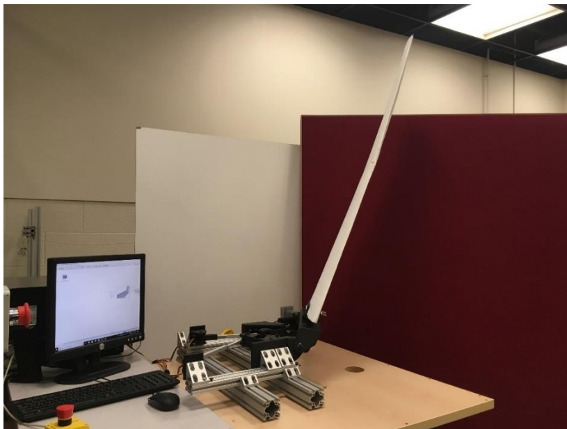
Figure 5-22: Prototype test setup with Winglet at 10°
