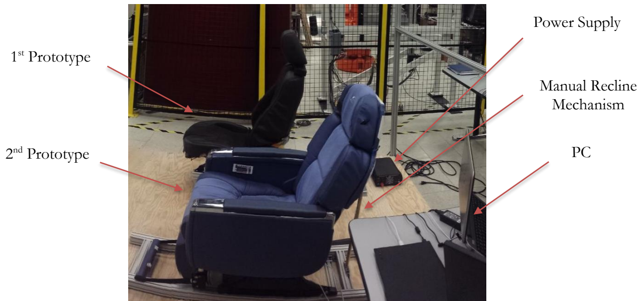
Figure 6-1: Experimental setup of seat prototypes.
