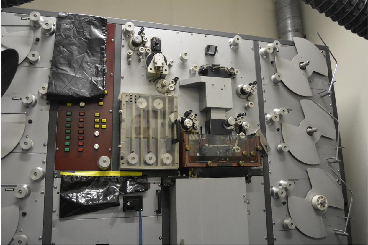
**Figure 4.** Andre Debris S.A. Paris optical step printer used to create the duplicate negative from the original nitrate at Haghefilm.
