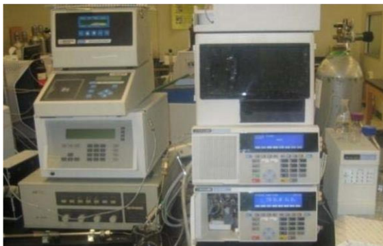
Figure 3.2. HPLC (model # 600 by Perkin Elmer) equipped with refractive index (Model # HP1047 A, Hewlett Packard).
