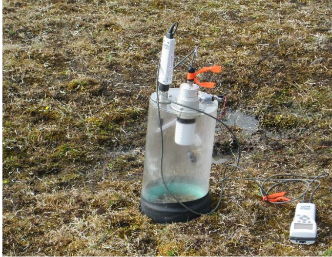
Figure 2: CO 2 Flux Static Chamber Apparatus for NEE Measurements
