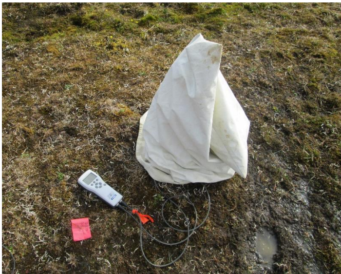
Figure 3: CO 2 Flux Static Chamber Apparatus for ER Measurements
