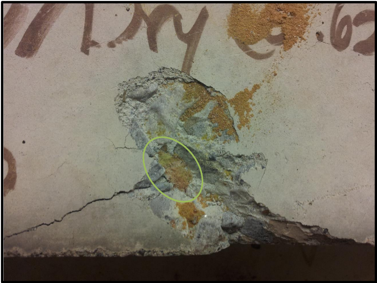
Figure 4.2.3: Image of Phase I Dolostone-0.62 specimen tested under dry conditions with hot/cold cycles of 150°C/23°C
