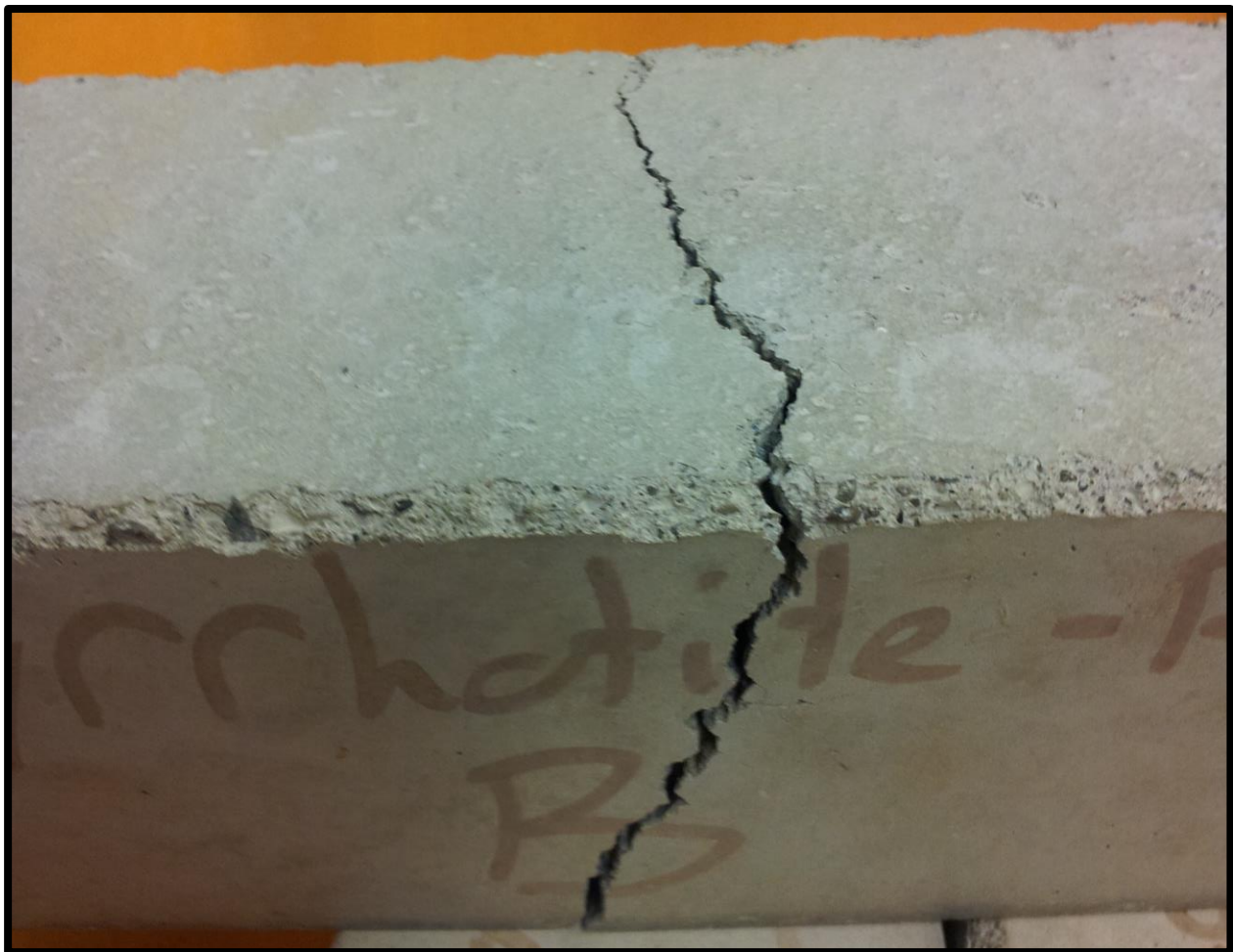
Figure 4.2.2: Image of Phase I Sulfide-0.45 sample tested under dry conditions with hot/cold cycles of 150°C/23°C
