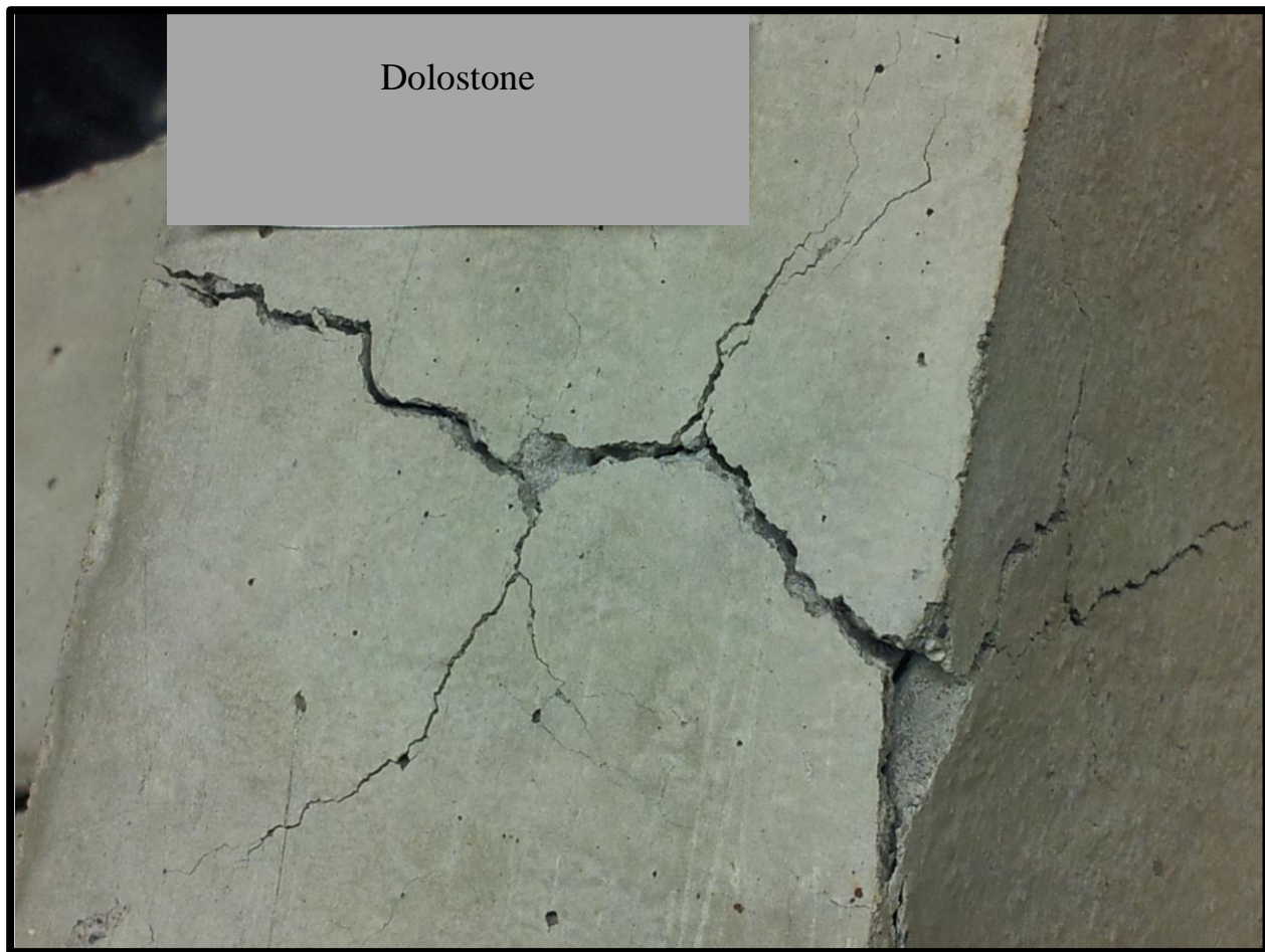
Figure 4.2.5: Image of severely cracked Phase I Dolostone-0.45 sample tested under dry conditions with hot/cold cycles of 150°C/23°C
