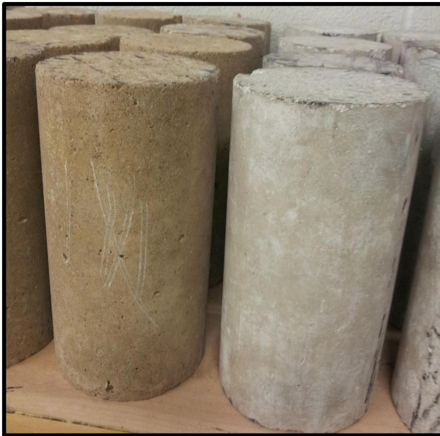
Figure 4.6.1: Cylinders tested under Phase III conditions, bleach soaked on left, lime solution soaked on the right; all samples have w/c=0.65 , were tested with 24-hour soaking at 23^{\circ}\text{C} twice a week, and 24-hours heating/drying to 60^{\circ}\text{C} twice a week
